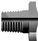
**KF**-British Standard BS21 (ISO 7-1), Internal pipe threads
