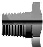
**F**-ANSI/ASME B1.20.1, Internal pipe threads
