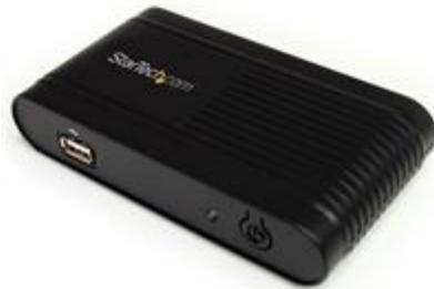
The WIFI2VGA VGA over Wi-Fi Adapter enables you to send a VGA signal (resolutions up to 1280x1024/720p), as well as the supporting audio from a laptop or desktop computer, to a remote projector or display over a wireless IP network.
