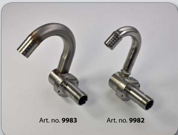
Low pressure swivel joints, suitable for hose reels in 1' 1/4" and 1' 1/2", with fixed fluid shaft and swivelling support, gooseneck assembly and hose tail connections ø 33 mm and ø 38 mm.
