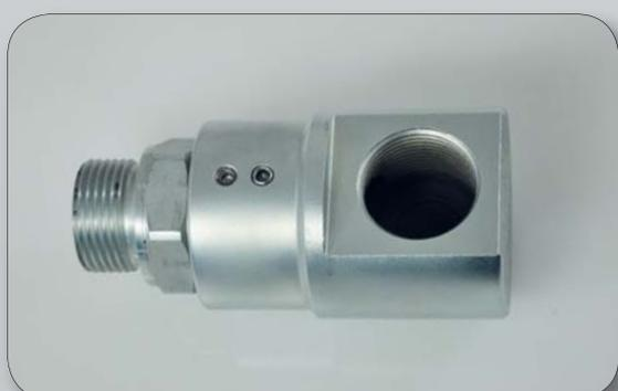
Swivel joint, 90° - type, with ball valve, self-lubricating. Body in galvanized steel, on demand also in stainless steel AISI 304. Connections (BSP): inlet F – outlet F.
