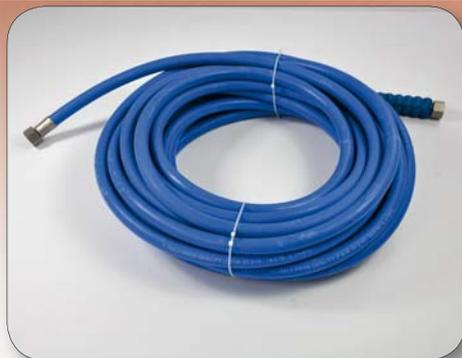
Low pressure synthetic rubber hoses with swaged female BSP connection threads (swivel nuts) in brass (on demand also in stainless steel), suitable for the use with **hot water** in food industry applications. Internal structure white, food industry – qualified synthetic rubber, coating in blue rubber highly resistant to abrasion, heat, ozone and atmospheric influences. Reinforcement with highly resistant synthetic cord. In accordance with FDA food industry standards.
