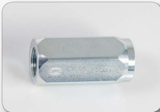
Non-return valve with high pressure gate valve, suitable for lubricants pipeworks. Body in galvanized steel, on demand also in stainless steel. Opening pressure 0.5 bar (on demand also 4 bar or 8 bar). Connections (BSP): inlet F – outlet F.
