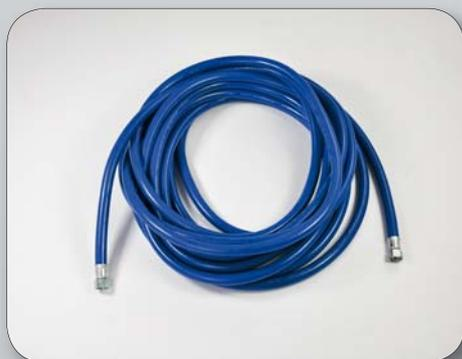
Low pressure, blue PVC – hoses with swaged female BSP connection threads (swivel nuts) in brass, suitable for the use with **compressed air and water** at low pressure. Reinforcement with highly break resistant polyester cord.
