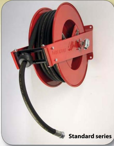
Automatic, spring – driven hose reel, standard series, in painted steel, including rubber hoses SAE 100 R1 AT with female connection threads, suitable for the supply of oil and antifreeze.
