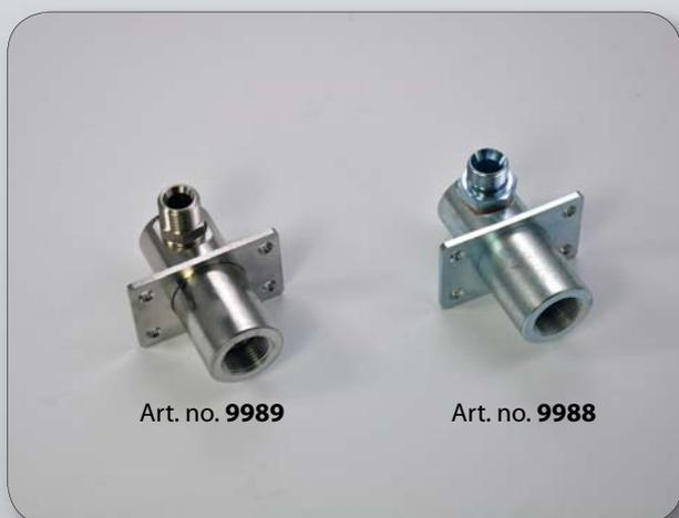
Interchangeable fluid shaft suitable for installation in hose reel series EVO in 1/2". They are available in galvanized and stainless steel AISI 304. In combination with the swivel joints of catalogue pages 224 and 225 they enable the use of a painted steel hose reel model also for fluids that require wetted parts in stainless steel (f. ex. water, AdBlue®/DEF/AUS32), just by changing the components which are in contact with the fluid.
