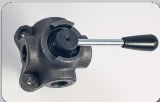
4-way flow diverter valve in cast iron, open center, with limited pressure drops. Made with 2 fixing holes Ø 8.5 mm.
