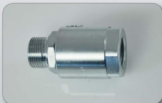
Swivel joint, straight type, with ball valve, self-lubricating. Body in galvanized steel, on demand also in stainless steel AISI 304. Connections (BSP): inlet F – outlet F.
