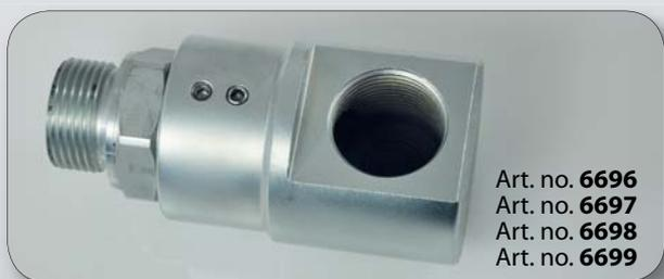
Swivel joint, 90° - type, with ball valve, self – lubricating. Body in galvanized steel, on demand also in stainless steel AISI 304. Connections (BSP): inlet F – outlet F.
