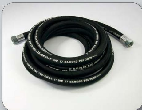
Low pressure rubber hoses in accordance with SAE 100 R6 – DIN EN 854, with swaged female BSP connection threads (swivel nuts), suitable for the supply of **diesel** and **petrol** at low pressure.
