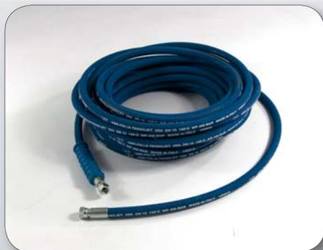
High pressure, **blue antistaining rubber hoses**, in accordance with SAE 100 R2AT, with swaged female BSP connection threads (swivel nuts), suitable for the supply of **water** at high pressure (f. ex. in combination with high pressure cleaners).
