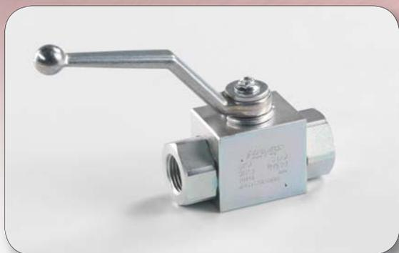
High pressure ball valve, with full port and lever handle, suitable for lubricants pipeworks. Body in galvanized steel. Connections (BSP): inlet F – outlet F.
