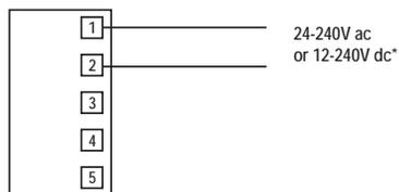
\*NOTE: Connection of dc power is without regard to polarity
