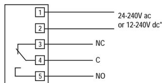
\*NOTE: Connection of dc power is without regard to polarity
