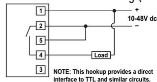
NOTE: This hookup provides a direct interface to TTL and similar circuits.
