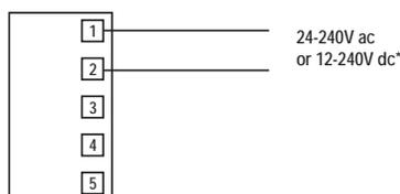
\*NOTE: Connection of dc power is without regard to polarity
