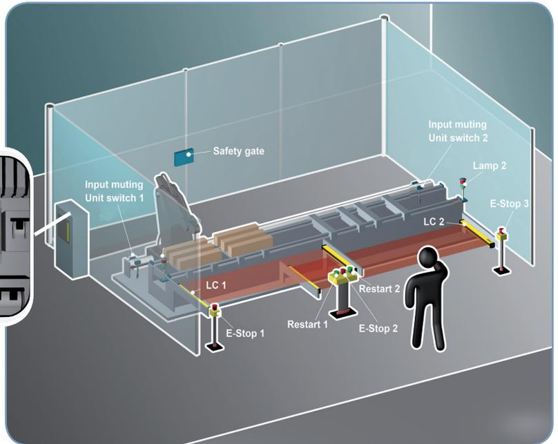
Total safety components: 2 safety light curtains - 2 restart buttons for the safety light curtains - 1 safety gate switch - 3 emergency push buttons.
