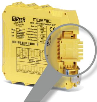
Mosaic MSC permits communication between the various units through a proprietary 5-way high-speed safety bus.
