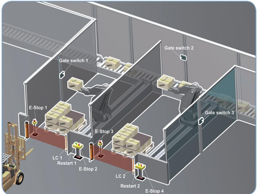
Total safety devices: 2 safety light curtains - 2 restart buttons for the safety light curtains - 3 safety gate switches - 4 emergency push buttons.
