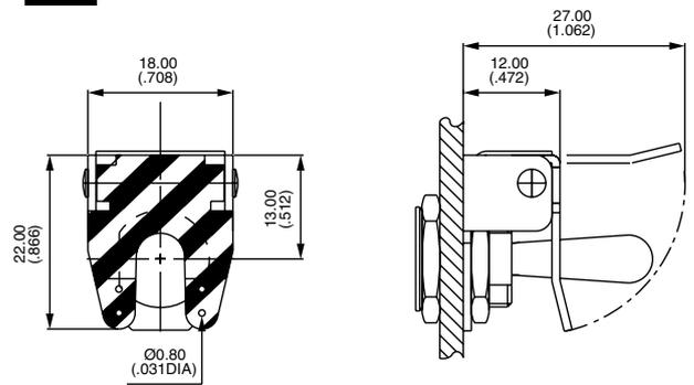
Plate features holes for wiring a seal.
