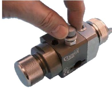
**13.** The fluid needle control knob is located at the rear of the gun body. However, like a Pressure fed hand gun the main fluid control should be carried out by the fluid Pressure and the Fluid Nozzle diameter.
