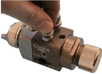
**12.** The atomizing air is controlled by the second ATOM valve
