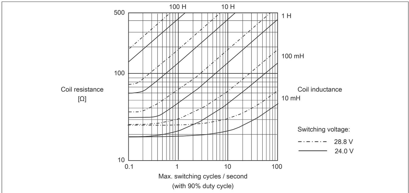
Environmental temperature: 60°C, all outputs with the same load.
