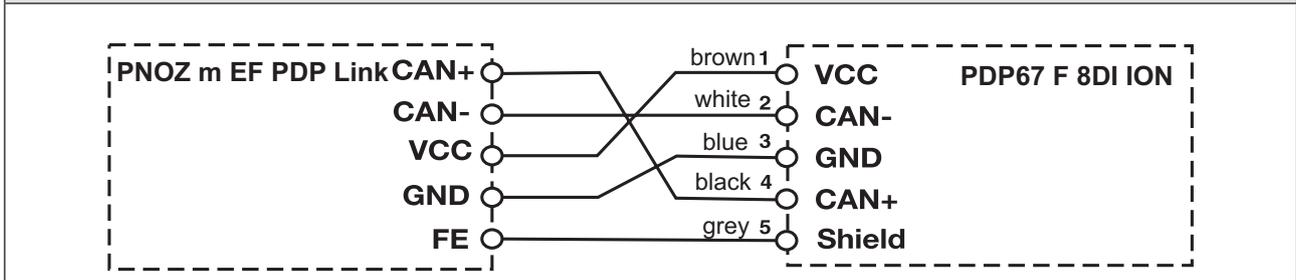
Connection when using the PSS SB BUSCABLE LC in conjunction with a Pilz self-assembly "PSS67 M12 connector" (see order reference in the Technical Catalogue)
