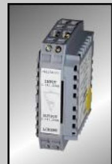
The galvanic separators CAL25IG are design to isolate current loops 0...4...20mA. No auxiliary power supply is required, there are easily integrated in existing current loops. It's a way to eliminate the ground loop or common mode problems.
