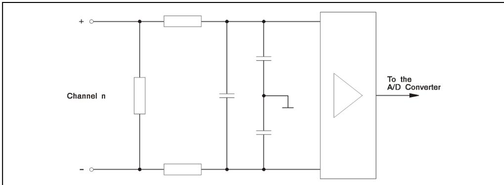
Figure 128: AI775 input circuit diagram
