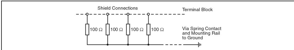
Figure 127: AI775 shielded connection
