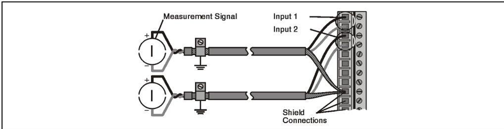
Figure 126: AI775 signal cable connection
