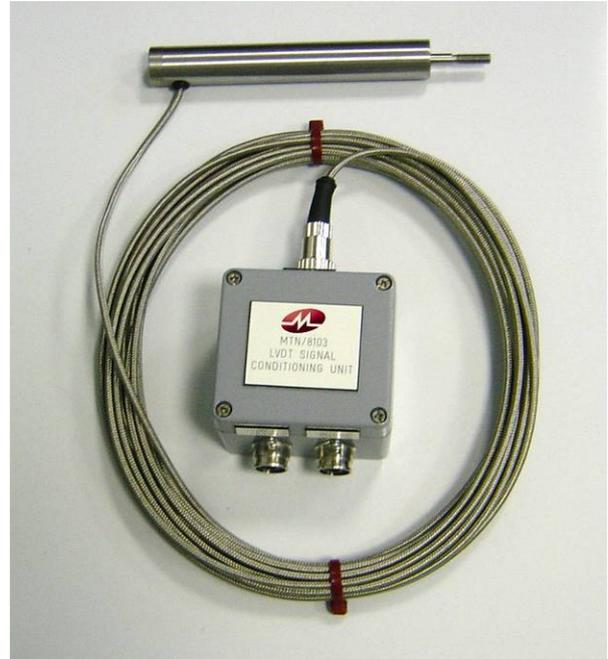
External signal conditioner in robust industrial enclosure with IP66 ingress protection
