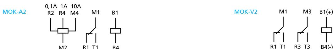
Selection of the range is made by connecting to the respective terminal.
