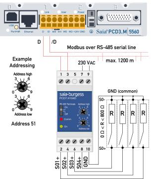
Note: If the S0-Modbus module is used in the Modbus as last device, then the sliding switch «RS485 Terminate» need to be in the position «On».
