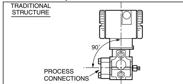
Figure 3. Vertical Mounting Showing Process Connections at 90 degrees
