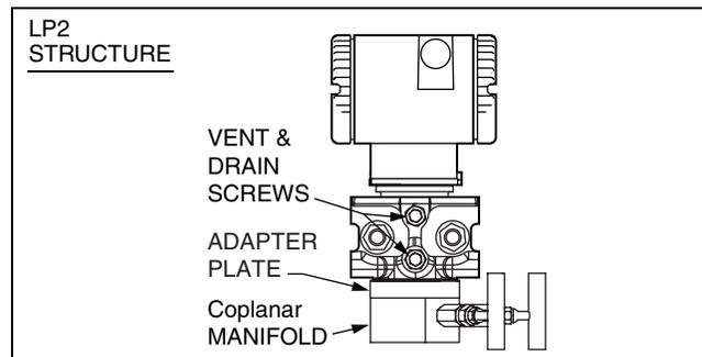
Figure 15. Adapter Mount to Existing Coplanar Manifold
