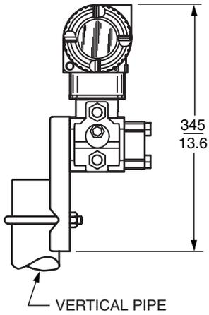
**TRANSMITTER WITH LOW PROFILE STRUCTURE LP2**
