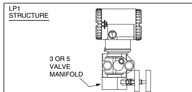
Figure 8. LP1 Shown Directly Mounted to Manifold
