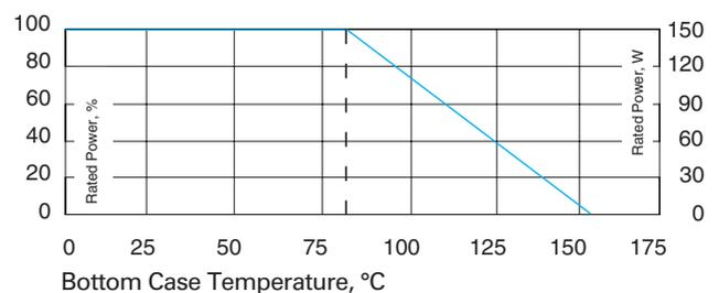
Derating (thermal resistance): 2.14 W/°K (0.47°K/W).
