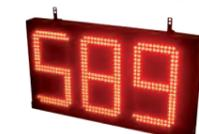
**Outdoor display with 3 digits,** indicating the number of parking spaces available, high-luminosity red LED. Digit height: 300 mm. Dimensions: 676mm x 381mm x 70mm. Consumption: 37W. IP54. Luminosity control via software. Aluminium casing. Communication: RS485. Input power: 230 V AC.
