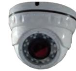
**Domo Camera** with autozoom 2.8-12mm and vandalproof for LPR each 3 parking spaces. 3MP resolution (H.264/H.265). IR cut filter with 30m range. External POE included. HD lens 1/2,9" SONY sensor CMOS low illumination.
