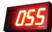
**Outdoor display with 3 digits,** indicating the number of parking spaces available, high-luminosity red LED. Digit height: 110 mm. Dimensions: 335mm x 209mm x 70mm. Consumption: 15W. IP54. Luminosity control via software. Aluminium casing. Communication: RS485. Input power: 230 V AC.
