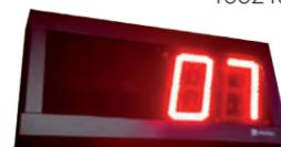
**Outdoor display with 2 digits,** indicating the number of parking spaces available, high-luminosity red LED. Digit height: 110 mm. Dimensions: 335mm x 209mm x 70mm. Consumption: 10W. IP54. Luminosity control via software. Aluminium casing. Communication: RS485. Input power: 230 V AC.
