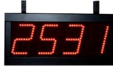
**Outdoor display with 4 digits,** indicating the number of parking spaces available, high-luminosity red LED. Digit height: 110 mm. Dimensions: 407mm x 209mm x 70mm. Consumption: 20W. IP54. Luminosity control via software. Aluminium casing. Communication: RS485. Input power: 230 V AC.
