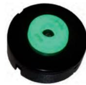
**Ultrasonic sensor and Indicator light on the same equipment,** for the detection and indication of occupancy status of the parking space. Power+data Connector and external light connector. Power supply: 24 Vdc. Consumption: 1.2 W. Communications: RS-485. Extended Temperature Range -10 to 50°C. Remote Configurable Firmware. Recommended installation height between 2.30 and 3.5 meters. Detection distance adjustable by software. It with Red-Green led indicator.
