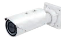
**Domo Camera** with autozoom 2.8-12mm and vandalproof for LPR by zone. 3MP resolution (H.264/H.265). IR cut filter with 60m range. External POE included. HD lens 1/2,9" SONY sensor CMOS low illumination.
