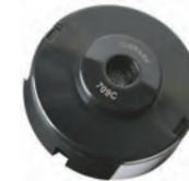
**Ultrasonic sensor** for the detection of occupancy status of the parking space. Power+data Connector and external light connector. Power supply: 24 Vdc. Consumption: 0.8 W. Communications: RS-485. Extended Temperature Range -10 to 50°C. Remote Configurable Firmware. Recommended installation height between 2.30 and 3.5 meters. Detection distance adjustable by software.
