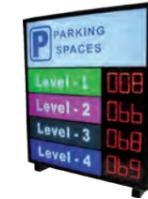
**Panel with information** about the capacity of the car park, per floor or overall. 2-3-4 digit displays. Input power: 24 V DC. Consumption: 2.5 - 4 W per panel. Communication: RS-485. Digit colour: amber - red. Brightness intensity adjustable by software.
