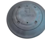
**Magnetic Field Surface Sensor** for the detection of occupancy status of the outdoor parking space. Power: Internal Batteries 14,4 Ah. RF Communications 868MHz. Coverage of 100m. Detection height of 0.5m. Extended Temperature Range -20 to 60°C. Remote Firmware configurable. IP67 protection. Shelf Life 5 years. Changeable batteries.
