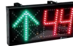
**Indoor display in mode: [2 digits + Cross/Arrow].** RGB LEDs with 120° angle. 8 predefined digit colors. Height digit 125 mm. Right/Left and Up/Down controllable arrow. Arrow: Green/Red and Cross: Red. Indication of free places and address. Display "FULL" or "000 Arrow/Cross". Power supply: 48-24 Vdc. Maximum consumption: 11 W. Communications: RS-485. Dimensions: 324 x 165,23 x 39 mm.
