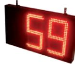
**Outdoor display with 2 digits,** indicating the number of parking spaces available, high-luminosity red LED. Digit height: 300 mm. Dimensions: 676mm x 381mm x 70mm. Consumption: 25W. IP54. Luminosity control via software. Aluminium casing. Communication: RS485. Input power: 230 V AC.
