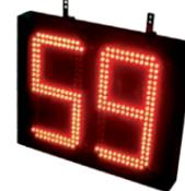
**Outdoor panel, indicating the number of parking spaces available, two digits, high-luminosity red LED.** Digit height: 200 mm. Dimensions: 514mm x 290mm x 70mm. Consumption: 25W. IP54. Luminosity control via software. Aluminium casing. Communication: RS485. Input power: 230 V AC.
