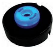
**Ultrasonic sensor and Indicator light on the same equipment,** for the detection and indication of occupancy status of the parking space. Power+data Connector and external light connector. Power supply: 24 Vdc. Consumption: 1.2 W. Communications: RS-485. Extended Temperature Range -10 to 50°C. Remote Configurable Firmware. Recommended installation height between 2.30 and 3.5 meters. Detection distance adjustable by software. It has led indicator Red-Blue (2000 mcd).
