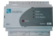
**Vehicle counting equipment.** Control unit for inductive loop, photocell or DPU pass detectors. Power supply: 24 Vdc. Consumption: 1 W + (Number of zones x 1,6 W). Communications via RS-485. 8 digital inputs for control of up to 4 pass-zones. Additional RS-485 input for control of up to 4 DPU. Incorporates 4 relay outputs for automation, depending on the occupation. Storage memory for the 4 pass-zone counters.
