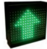
**Display Cross/Arrow, address indication of Free Places.** Arrow Color: Green-Red. 10 arrow positions. Brightness intensity adjustable by software. Power supply: 24 Vdc. Consumption: 2.5 W. Communications: RS-485. Height Arrow 120 mm. Dimensions: 164 x 165,23 x 39 mm.
