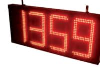
**Outdoor display with 4 digits,** indicating the number of parking spaces available, high-luminosity red LED. Digit height: 200 mm. Dimensions: 584mm x 290mm x 70mm. Consumption: 45W. IP54. Luminosity control via software. Aluminium casing. Communication: RS485. Input power: 230 V AC.
