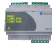
**Parking Concentrator,** with Management and Information storage capacity. Control of Equipment through Bus RS485, for Counting Systems, Energy Efficiency, Electrical Car Charging Stations and Automation. Incorporates a CirPark Scada embedded limited distribution. It has 4 digital inputs and 4 relay outputs. 10BaseT / 100Base TX Ethernet Port. 230 Vac power supply.
