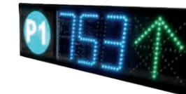
**Indoor display in mode: [Symbol + 3 digits + Cross/Arrow].** RGB LEDs with 120° angle. Customizable symbol with backlit vinyl. 8 predefined digit colors. Height digit 125 mm. Right/Left and Up/Down controllable arrow. Arrow: Green/Red and Cross: Red. Indication of free places and address. Display "FULL" or "000 Arrow/Cross". Power supply: 48-24 Vdc. Maximum consumption: 22,5 W. Communications: RS-485. Dimensions: 564 x 165,23 x 39 mm.
