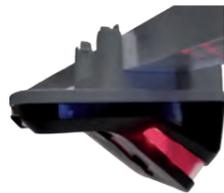
**Front-end Ultrasonic Sensor and RGB led indicator,** for the detection and indication of the occupancy status of the parking space. High brightness RGB led indicator Power: 24/48 Vdc. Consumption: 1.5 W. Communications: RS-485. It has connector for Power+data. Extended Temperature Range -20 to 60°C. Remote Configurable Firmware. Sensing distance and brightness intensity adjustable by software. Recommended installation height between 2.10 and 3.5 meters. IP54 Protection.
