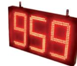
**Outdoor display with 3 digits,** indicating the number of parking spaces available, high-luminosity red LED. Digit height: 200 mm. Dimensions: 514mm x 290mm x 70mm. Consumption: 35W. IP54. Luminosity control via software. Aluminium casing. Communication: RS485. Input power: 230 V AC.
