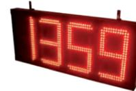
**Outdoor display with 4 digits,** indicating the number of parking spaces available, high-luminosity red LED. Digit height: 300 mm. Dimensions: 676mm x 381mm x 70mm. Consumption: 48W. IP54. Luminosity control via software. Aluminium casing. Communication: RS485. Input power: 230 V AC.
