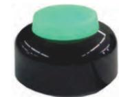
**Parking space occupancy status indicator,** with 360° vision, Red-Green color (2000 mcd). Power supply: 24 Vdc. Consumption: 0.7 W. Direct connection to the SP series detection sensor. Adjustable brightness intensity.
