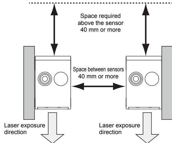
The LS series performs measurements by emitting a parallel laser beam and receiving the reflected light. During measurement, ensure that the laser beam and reflected light is not blocked by the target object.
