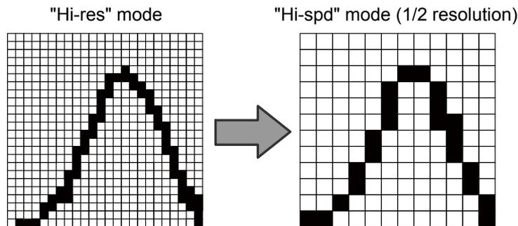
Figure: Difference in resolution attributable to the camera mode (example)
