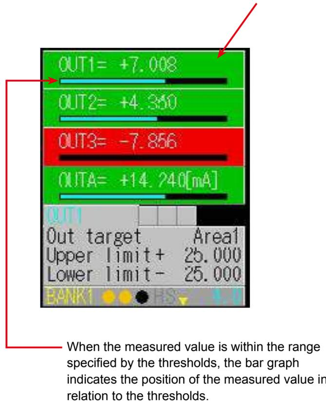
When the measured value is within the range specified by the thresholds, the bar graph indicates the position of the measured value in relation to the thresholds.
