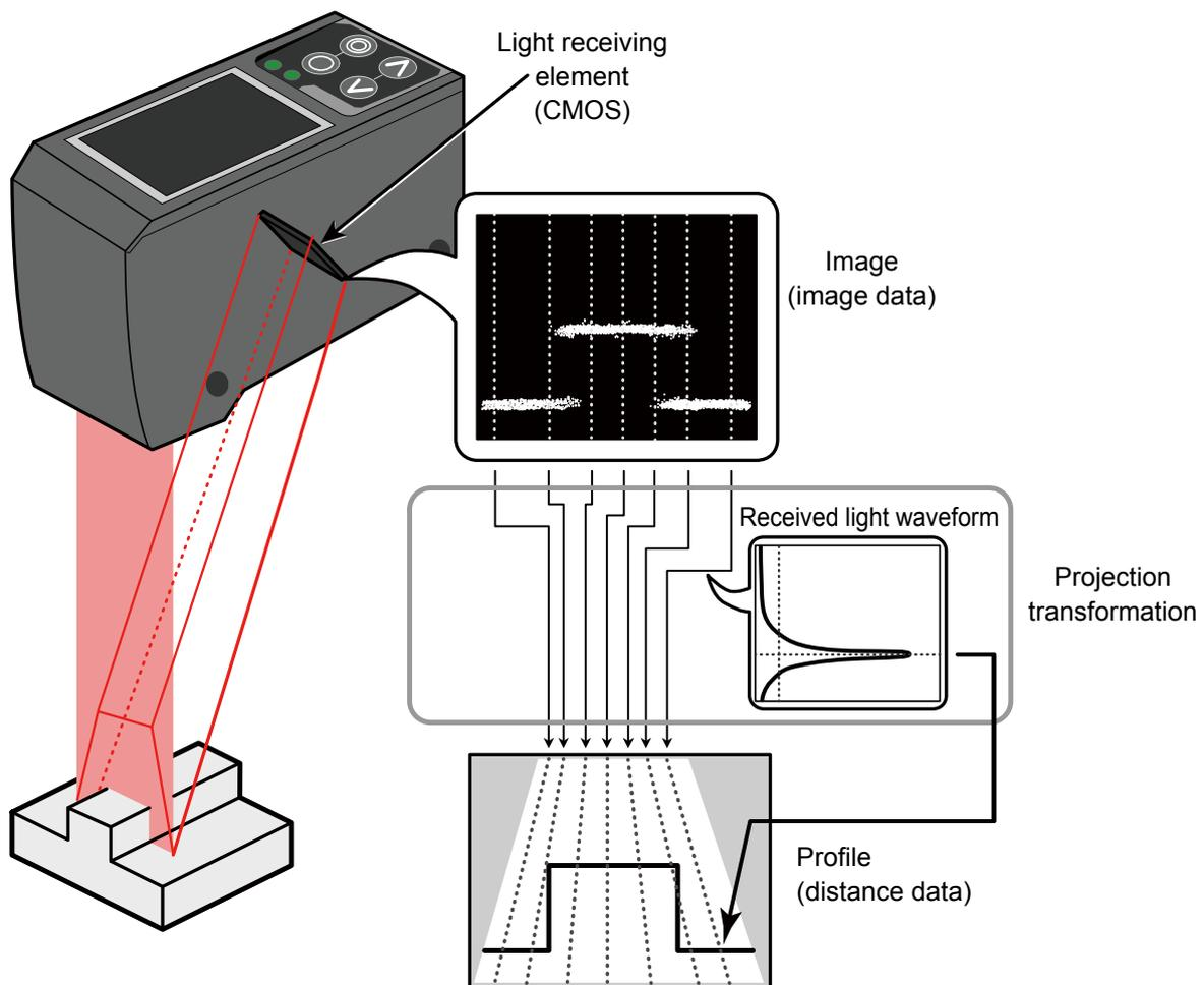
Figure: Schematic diagram of LS series measurement
