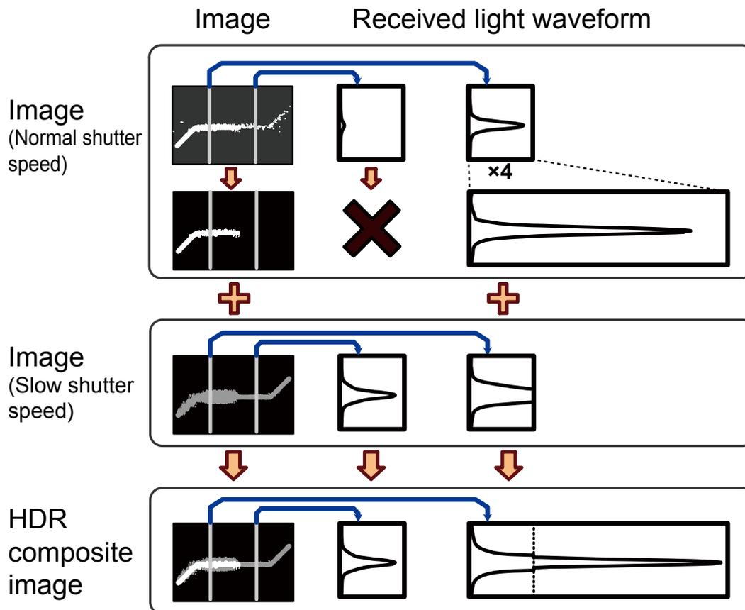
Adding the two images together makes it possible to measure any part of the resultant image with the appropriate amount of light.
