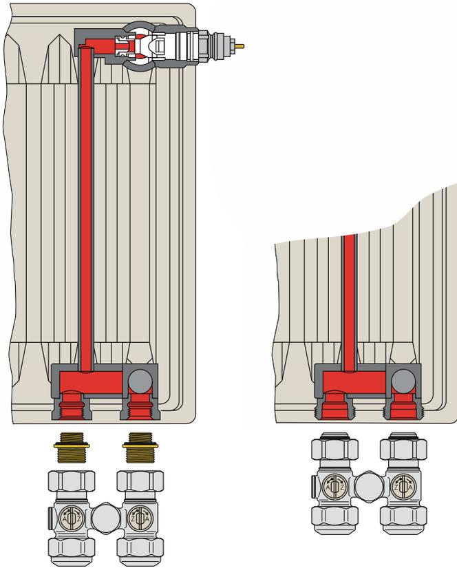
This valves are installed on a particular kind of panel radiators, featuring both the connections at the bottom and an inner pipe, invisible from outside, providing the flow medium to the upper valve.
