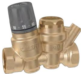
Thermostatic regulator for domestic hot water recirculation circuits. Fitted for automatic or controlled thermal disinfection function. With pocket for temperature gauge. **CR** "low lead" dezincification resistant alloy body. Female connections. Max. working pressure: 10 bar. Adjustment temperature range: 35–60°C.
