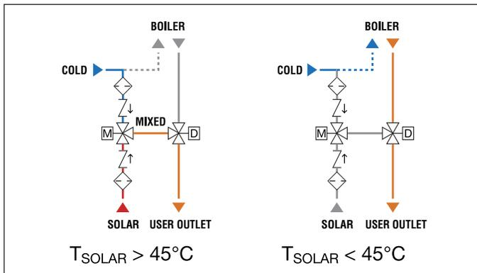
Solar storage-to-boiler connection kit, **without thermal integration**. Consisting of:
