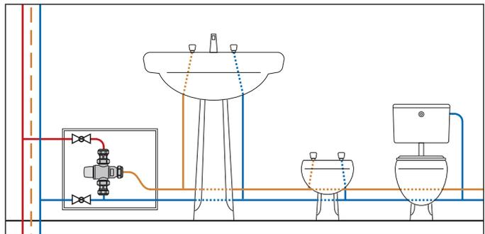
Application diagram of mixing valve 5213 series with distribution group
