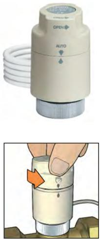
Thermo-electric actuator. With manual opening and position indicator. For valves 338, 339, 401, 402, 425, 426, 421, 422, 455, 456, 220, 221, 222, 223, 224, 225, 226 and 227 series. Normally closed. **With auxiliary microswitch.** Supply: 230 V (ac) or 24 V (ac)/(dc). Power consumption: 3 W. Starting current: ≤ 1 A. Starting current (656344/54): ≤ 250 mA. Auxiliary microswitch contact rating: 0,8 A (230 V). Ambient temperature range: 0–50°C. Protection class: IP 40. Cable length: 80 cm.
