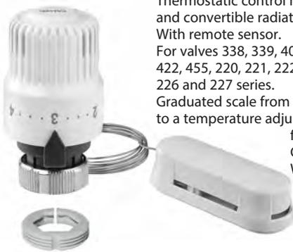
Thermostatic control head for thermostatic and convertible radiator valves. With remote sensor. For valves 338, 339, 401, 402, 425, 426, 421, 422, 455, 220, 221, 222, 223, 224, 225, 226 and 227 series. Graduated scale from \* to 5 corresponding to a temperature adjustment range from 7°C to 28°C. Capillary length: 2 m. With adapter.
