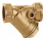
Y-strainer, for backflow preventers 573 and 574 series. Bronze body, 1/2"-2": PN 16, 2 1/2" - 3": PN 10. Female connections. Temperature range: -20-110°C. Max. percentage of glycol: 30%. Strainer in stainless steel stretched plate.
