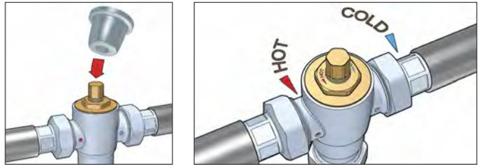
Application diagram of mixing valve 5213 series at point of use
