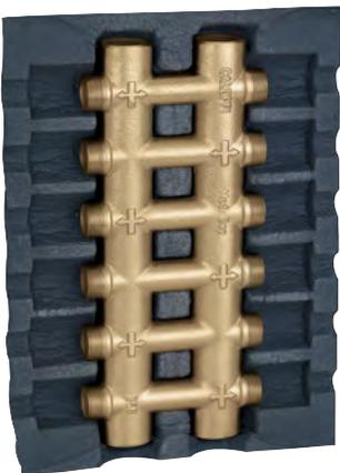
Cast monoblock dual distribution manifold. For heating and air conditioning systems. **With insulation.** Max. working pressure: 10 bar. Temperature range: 0–100°C. Main centre distance: 60 mm. Outlet centre distance: 40 mm.
