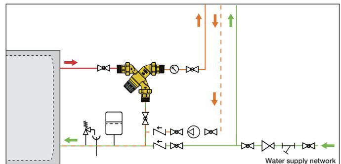
CONTROL UNIT FOR DOMESTIC HOT WATER TEMPERATURE
