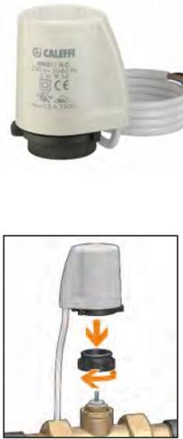
Thermo-electric actuator. With opening position indicator. **Quick-coupling installation, with a clip adapter.** For valves 338, 339, 401, 402, 425, 426, 421, 422, 455, 456, 220, 221, 222, 223, 224, 225, 226 and 227 series. Normally closed. **With auxiliary microswitch.** Supply: 230 V (ac) or 24 V (ac)/(dc). Auxiliary microswitch contact rating: 0,8 A (230 V). Power consumption: 3 W. Starting current: ≤ 1 A. Ambient temperature range: 0–50°C. Protection class: IP 54. Cable length: 80 cm.
