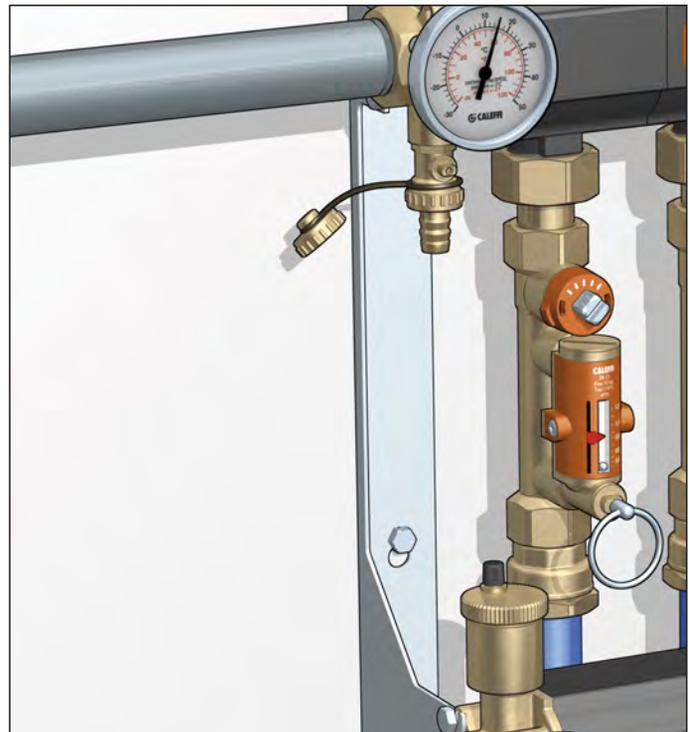
The use of a flow meter greatly simplifies the process of system balancing, since the flow rate can be measured and controlled at any time and there is no need for differential pressure gauges or reference charts.
