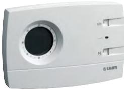
Digital chrono-thermostat, with battery supply. Daily or weekly programmable clock. 2 temperature levels + anti-freeze. Fitted for phone programmer. 30-minute minimum programme. Output contact: 8 (2) A. Protection class: IP 30.
