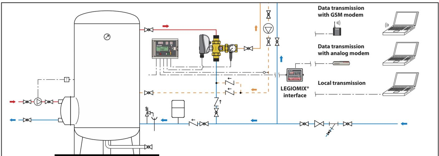
UNIT FOR TEMPERATURE CONTROL AND THERMAL DISINFECTION
