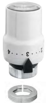
Thermostatic control head for radiator valves. Built-in sensor with liquid-filled element. With LCD type ambient temperature indicator. For valves 338, 339, 401, 402, 455, 220, 221, 222, 223, 224, 225, 226 and 227 series. Graduated scale from \* to 5 corresponding to a temperature adjustment range from 7°C to 28°C. Room temperature indicator range: 16–26°C. With adapter.
