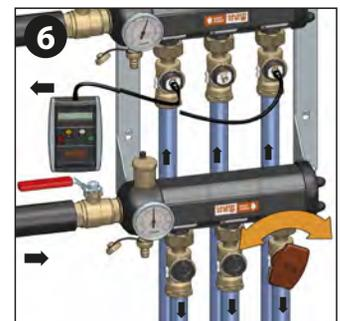
During the flow rate measurement, the sensor creates no significant head losses and therefore causes no significant changes in the actual flow rate.
