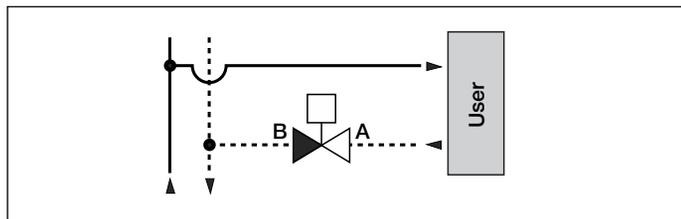
3-way valve installed on the flow with diverting position and ON/OFF use mode
