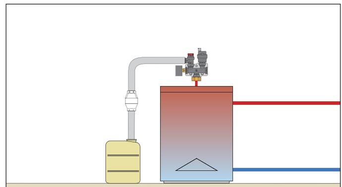
MULTIFUNCTION DEVICE IN COMPOSITE WITH DIRT SEPARATOR AND STRAINER
