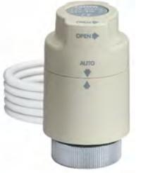
Thermo-electric actuator. With manual opening and position indicator. For distribution manifolds 662 and 663 series. Normally closed. **With auxiliary microswitch.** Supply: 230 V (ac) or 24 V (ac)/(dc). Power consumption: 3 W. Starting current: ≤ 1 A. Starting current (656344/54): ≤ 250 mA. Auxiliary microswitch contact rating: 0,8 A (230 V). Ambient temperature range: 0–50°C. Protection class: IP 40. Cable length: 80 cm.
