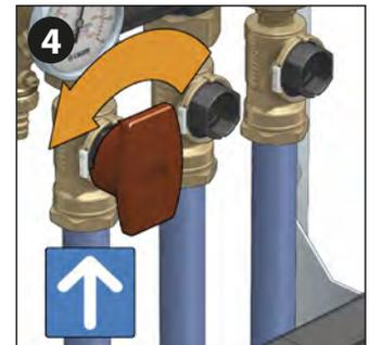
5. After carrying out these operations on all the outlets, it is possible to connect the electronic measurer to the sensor of the first branch and measure the corresponding flow rate. The flow rate is adjusted by regulating, with the special knob, the shut-off valve on the return manifold in correspondence with the same circuit until the instrument indicates the design setting.
