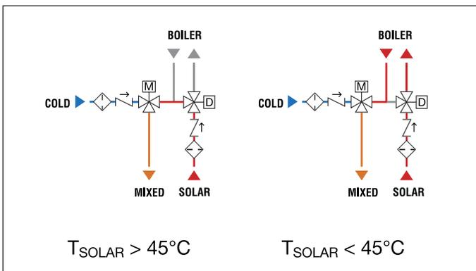
Application diagram of SOLARINCAL kit 265 series
