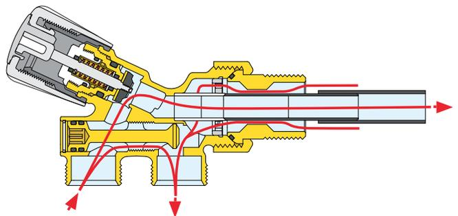
Flow and return connections can be inverted
