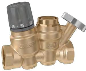
Thermostatic regulator for domestic hot water recirculation circuits. Complete with automatic thermostatic thermal disinfection function. With temperature gauge for circuit temperature check. **CR** "low lead" dezincification resistant alloy body. Female connections. Max. working pressure: 10 bar. Adjustment temperature range: 35–60°C. Disinfection temperature: 70°C.
