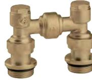
Differential by-pass for dual distribution manifolds 356 and 357 series. 3/8" connection for automatic air vent. Fixed differential by-pass setting: 20 kPa (2000 mm w.g.). Max. working pressure: 10 bar. Temperature range: -10–110°C.
