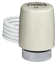
Thermo-electric actuator. For valves 338, 339, 401, 402, 425, 426, 421, 422, 455, 456, 220, 221, 222, 223, 224, 225, 226 and 227 series. Normally closed. **With auxiliary microswitch.** Supply: 230 V (ac) or 24 V (ac)/(dc). Auxiliary microswitch contact rating: 0,8 A (230 V). Power consumption: 3 W. Starting current: ≤ 1 A. Ambient temperature range: 0–50°C. Protection class: IP 44 (vertical stem). Cable length: 80 cm.
