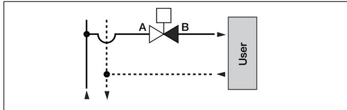
2-way valve installed on the return
