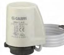
Thermo-electric actuator with low power consumption. With opening position indicator. **Quick-coupling installation, with a clip adapter.** For distribution manifolds 662 and 663 series. Normally closed. **With auxiliary microswitch.** Supply: 230 V (ac) or 24 V (ac)/(dc). Auxiliary microswitch contact rating: 0,8 A (230 V). Power consumption: 3 W. Starting current: ≤ 250 mA. Ambient temperature range: 0–50°C. Protection class: IP 54. Cable length: 80 cm.
