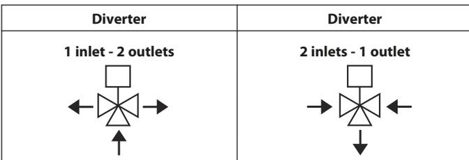
Operating diagram of valves 638 series - "L" drilling
