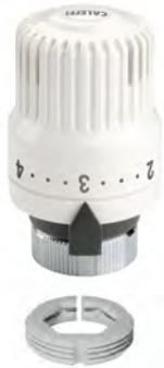
Thermostatic control head for convertible radiator valves. Built-in sensor with liquid-filled element. For valves 338, 339, 401, 402, 425, 426, 421, 422, 455, 220, 221, 222, 223, 224, 225, 226 and 227 series. Graduated scale from \* to 5 corresponding to a temperature adjustment range from 7°C to 28°C. With adapter.
