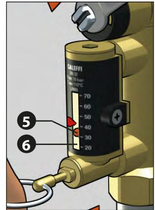
4. After completing the balancing, release the ring (2) of the flow meter obturator that, thanks to an internal spring, will automatically go back into the closed position.
