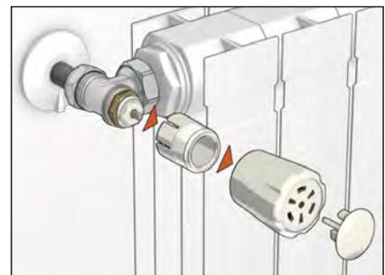
Lift the special control ring nut of the pre-setting device and turn the control stem to select the required position on the graduated scale.
