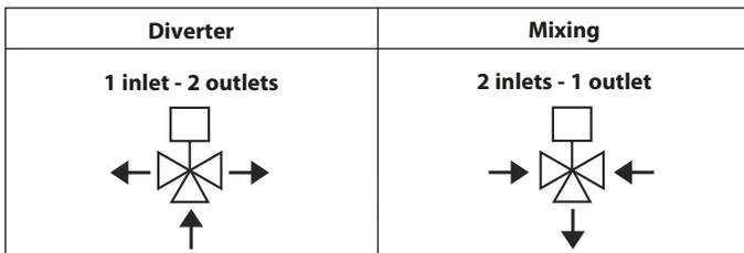
Operating diagram of valves 638 series - "T" drilling
