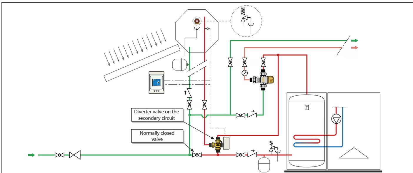
ANTI-SCALD THERMOSTATIC AND TEMPERING MIXING VALVES
