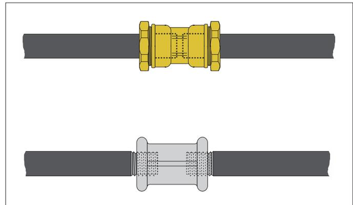
In order to avoid corrosion, which is typical when traditional threaded sleeves are used (see diagram in grey colour), the application of the **Steel** series fittings (see diagram in yellow colour) allows piping to keep the complete galvanisation.
