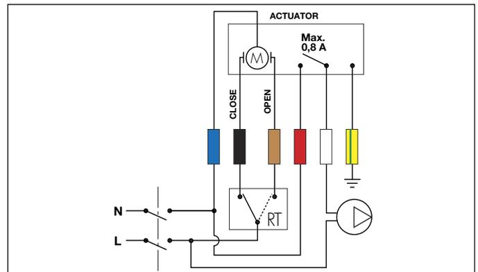
MOTORIZED THREE-WAY BALL DIVERTER VALVES
