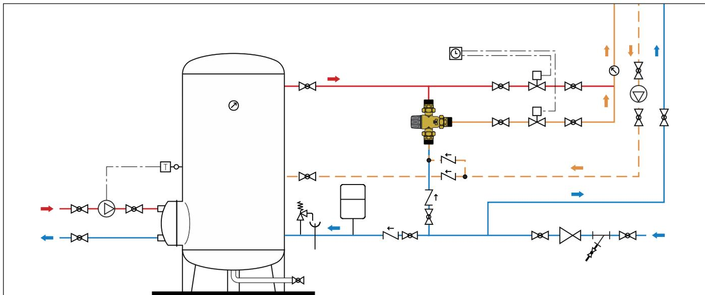
**THERMOSTATIC MIXING VALVE FOR MEDIUM-LARGE APPLICATIONS**
