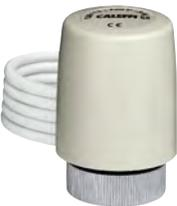
Thermo-electric actuator. For distribution manifolds 662 and 663 series. Normally closed. **With auxiliary microswitch.** Supply: 230 V (ac) or 24 V (ac)/(dc). Auxiliary microswitch contact rating: 0,8 A (230 V). Power consumption: 3 W. Starting current: ≤ 1 A. Ambient temperature range: 0–50°C. Protection class: IP 44 (vertical stem). Cable length: 80 cm.
