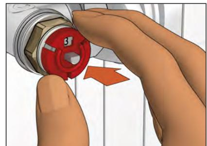
Position the manual knob, thermostatic control head or thermo-electric actuator on the valve.
