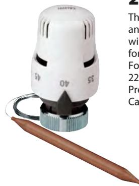
Thermostatic control head for thermostatic and convertible radiator valves; with contact probe, for medium temperature limiting. For valves 220, 221, 222, 223, 224, 225, 226, 227, 338, 339, 401, 402 and 455 series. Pre-set temperature scale. Capillary length: 2 m.
