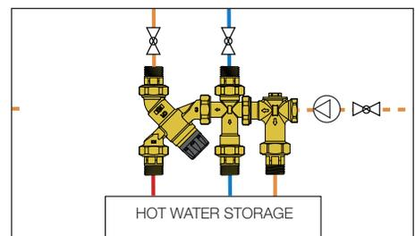
THERMOSTATIC MIXING VALVES FOR MEDIUM-LARGE APPLICATIONS
