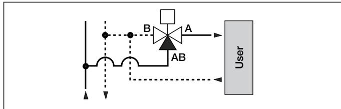
3-way valve installed on the return with mixing position and ON/OFF use mode
