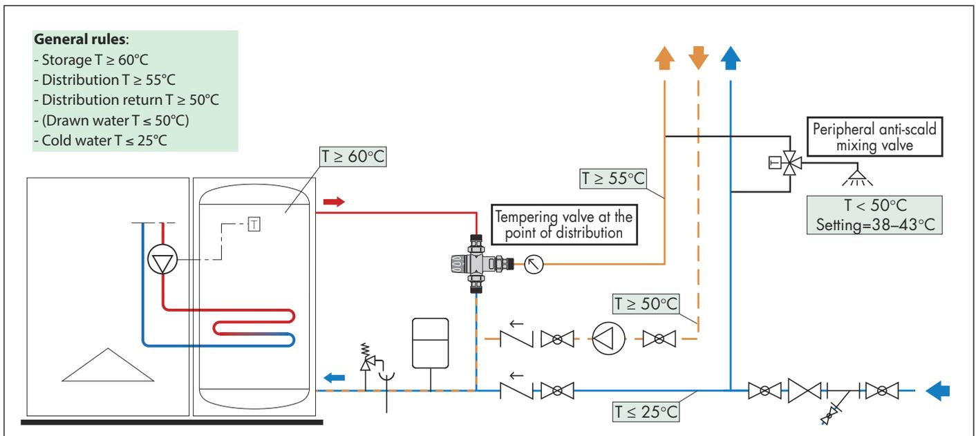
ANTI-SCALD THERMOSTATIC MIXING VALVES FOR INSTALLATION AT THE POINT OF USE
