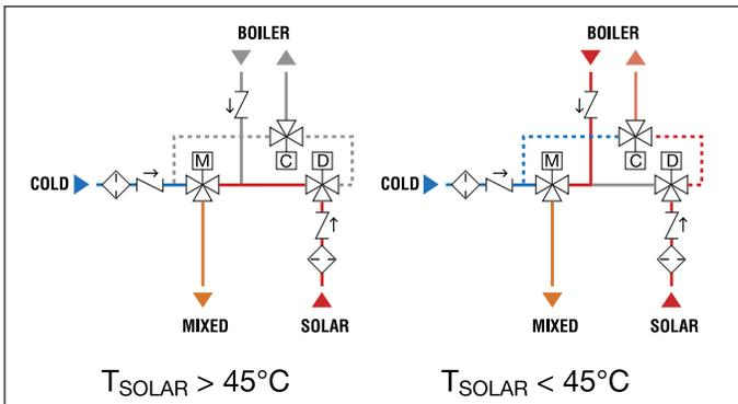
Solar storage-to-boiler connection kit, **with thermal integration**. Consisting of:
