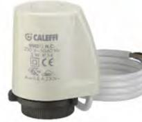
Thermo-electric actuator. With opening position indicator. **Quick-coupling installation, with a clip adapter.** For distribution manifolds 662 and 663 series. Normally closed. **With auxiliary microswitch.** Supply: 230 V (ac) or 24 V (ac)/(dc). Auxiliary microswitch contact rating: 0,8 A (230 V). Power consumption: 3 W. Starting current: ≤ 1 A. Ambient temperature range: 0–50°C. Protection class: IP 54. Cable length: 80 cm.
