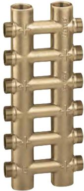
Cast monoblock dual distribution manifold. For heating and air conditioning systems. Max. working pressure: 10 bar. Temperature range: -10–110°C. Main centre distance: 60 mm. Outlet centre distance: 40 mm.
