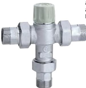
Thermostatic mixing valve, adjustable with knob, with check valves and strainers at the inlets. Enhanced thermal performance device with anti-scald safety function.
