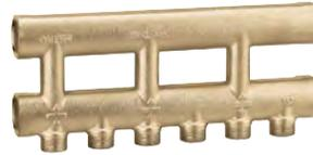
Single sided cast monoblock dual distribution manifold. For heating and air conditioning systems. Max. working pressure: 10 bar. Temperature range: -10–110°C. Main centre distance: 60 mm. Outlet centre distance: 40 mm.
