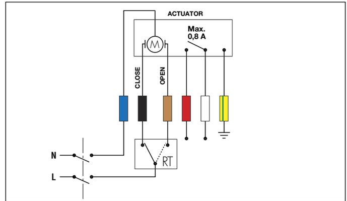
Connection diagram - with ON-OFF switch device
