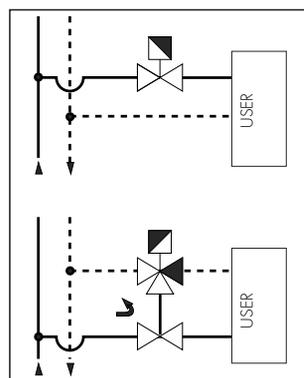
Wiring diagram for piston zone valves 632 and 633 series with thermo-electric actuator
