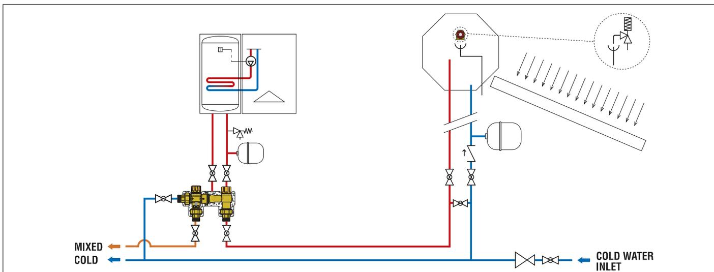
SOLAR STORAGE-TO-BOILER THERMOSTATIC CONNECTION KIT
