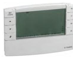
Digital room chrono-thermostat. **4 operating programmes with ON/OFF spark advance.** Weekly programmable clock. Fitted for phone programmer. 3 temperature levels + anti-freeze. 30-minute minimum programme. ON/OFF function with adjustable differential from 0,2 to 2°C or proportional. SUMMER - WINTER switch. Adjustable temperature with 0,1°C steps. 1 changeover switch output contact: 8 (2) A. Protection class: IP 30.
