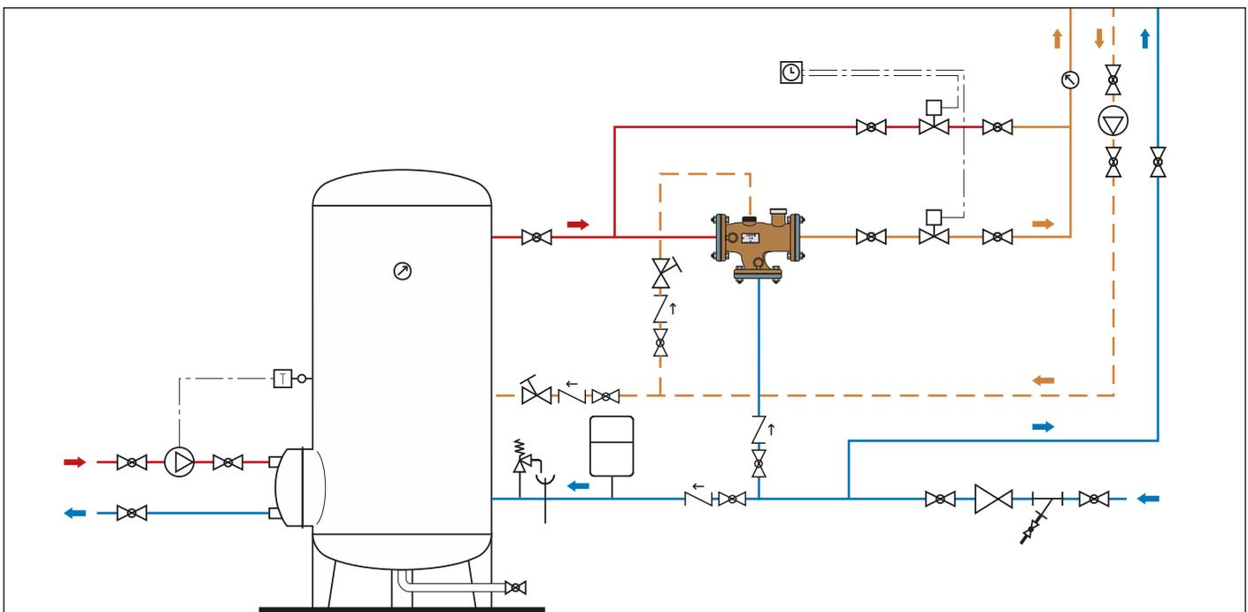
**ELECTRONIC MIXING VALVE WITH PROGRAMMABLE THERMAL DISINFECTION**
