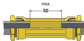
Allows pipe repairs
