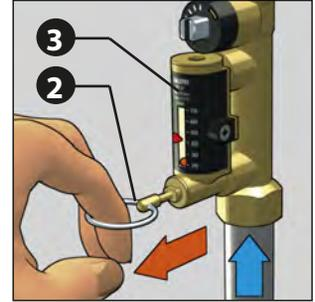
3. Keeping the obturator open, apply a wrench on the control stem of the valve (4) to adjust the flow rate. It is indicated by a metal ball (5) that runs inside a transparent guide (6) marked by a graduated scale in l/min.
