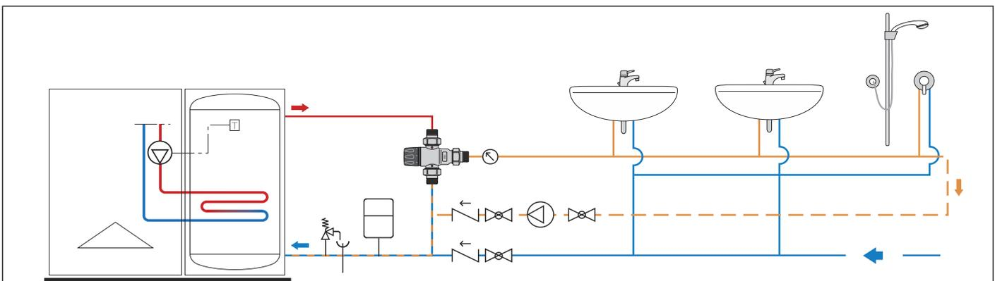
TEMPERING VALVE FOR INSTALLATION AT THE POINT OF DISTRIBUTION
