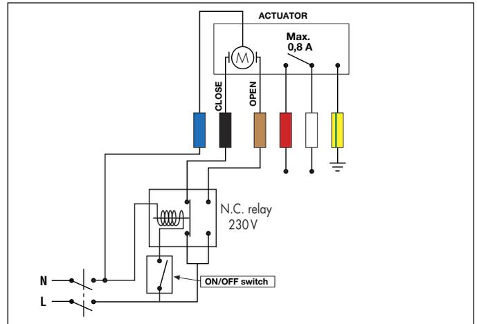
Pump disconnection diagram when no zone is in operation.
