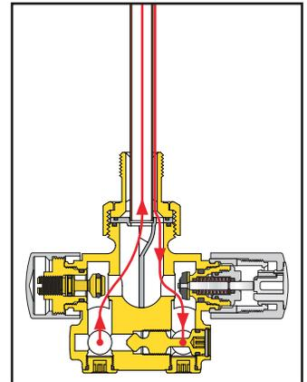
Flow and return connections can be inverted by means of the rotation of the specific deflector.
