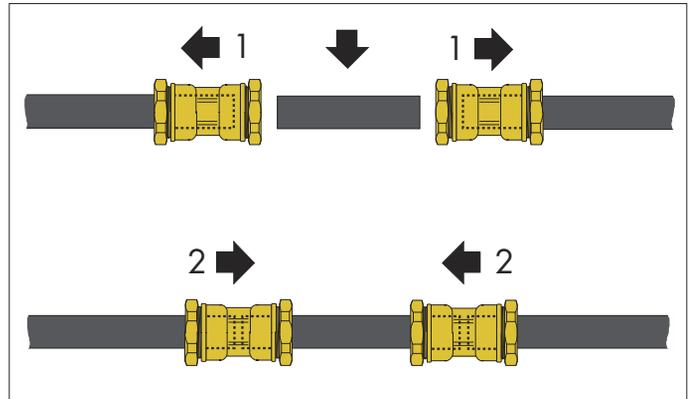
Example of repair with the insertion of a supplementary sleeve.
