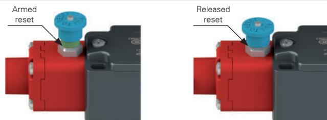
If the tension indicator is in the green area, the electrical safety contacts can be closed by pulling the blue knob. The reset status can be identified quickly by the green ring under the blue knob.
