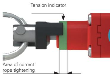
All switches are provided with a green ring that shows the area of the correct tightening of the rope. The installer has only to tighten the rope until the black indicator will be in the middle of the green area. With this setting, the switch can be reset by pulling the blue knob to close the electrical safety contacts.
