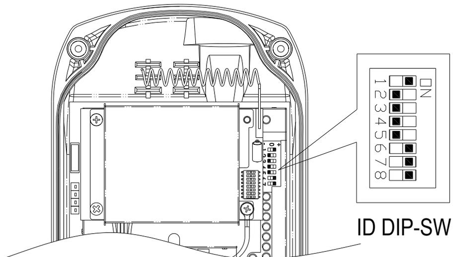
Set the ID codes needed with the dip-switch on the decoder board. For example: the ID codes set above → 10000111.
