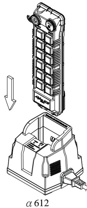
**NOTE!!! THE RECHARGEABLE BATTERIES HAVE TO BE RECHARGED WITHIN 6 MONTHS AFTER THE MANUFACTURING DATE.**
