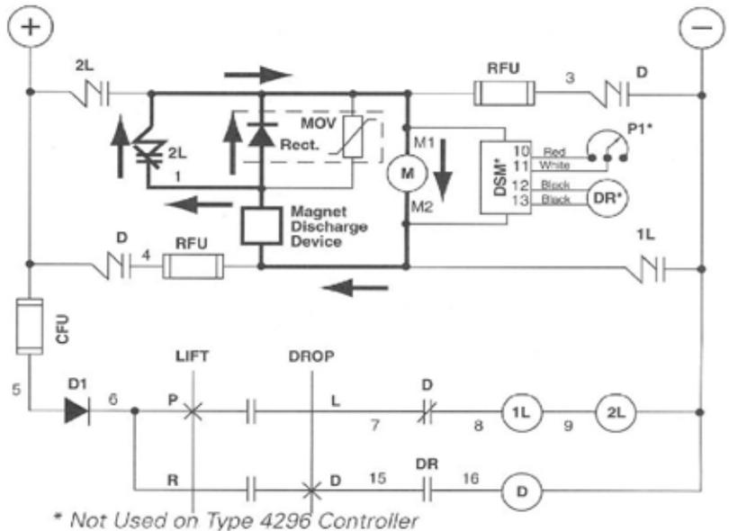
**Figure 5 — Schematic Diagram Reverse Current Cycle, 230V DC**
