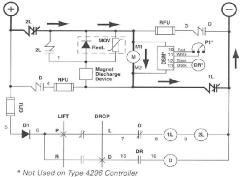
**Figure 4 — Schematic Diagram Priamy Discharge Cycle, 230V DC**
