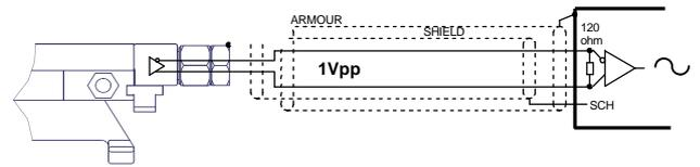
In case of cable extension, the electrical connection between the body of the connectors must be ensured.
