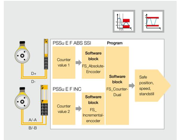
Safe speed, safe position – with two encoders.
