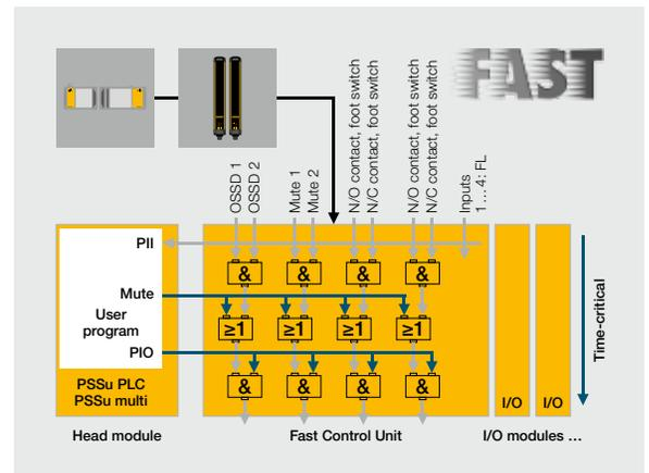
Signals are forwarded directly and rapidly. The user program has read and write access.
