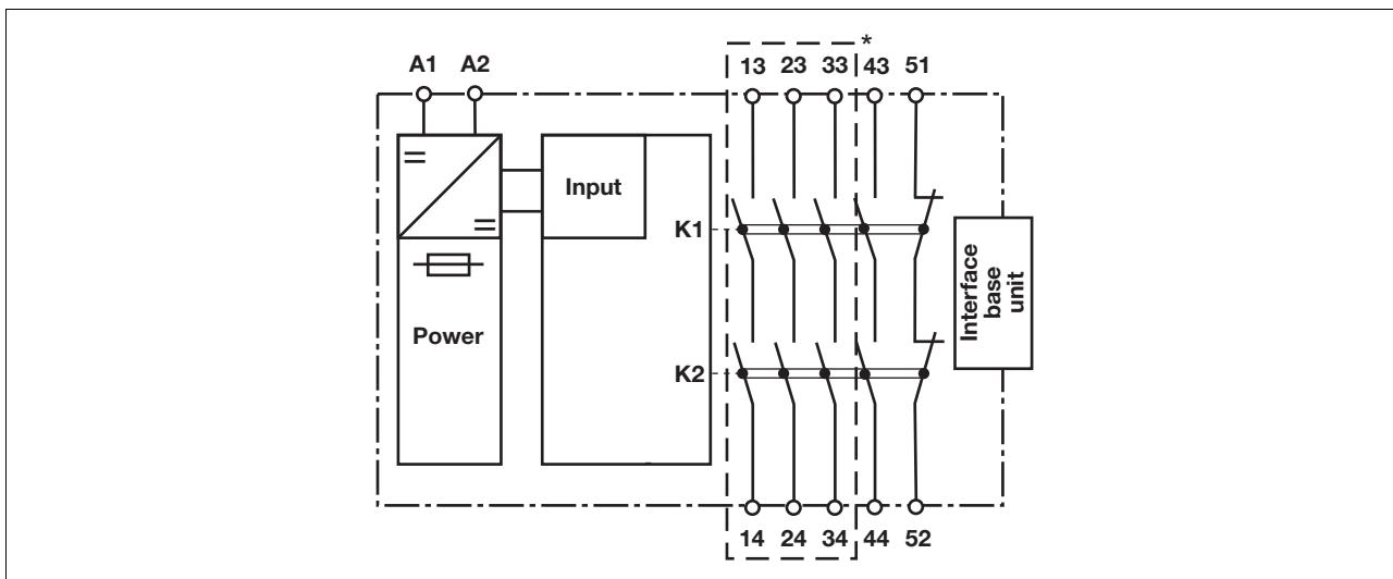
\* Safe separation in accordance with EN 60947-1, 6 kV
