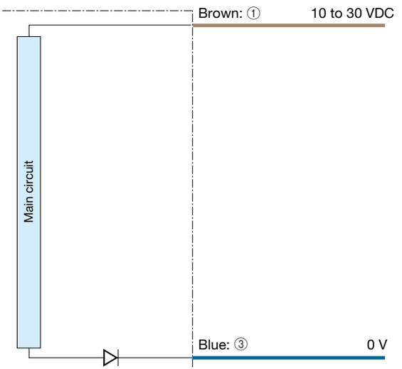
\*For the universal voltage type, add 24 to 240 VAC / 24 to 240 VDC to the brown wire and blue wire. (No polarity)
