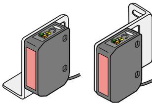
Tighten the sensor mounting screws with a tightening torque of no more than 0.5 N·m.
