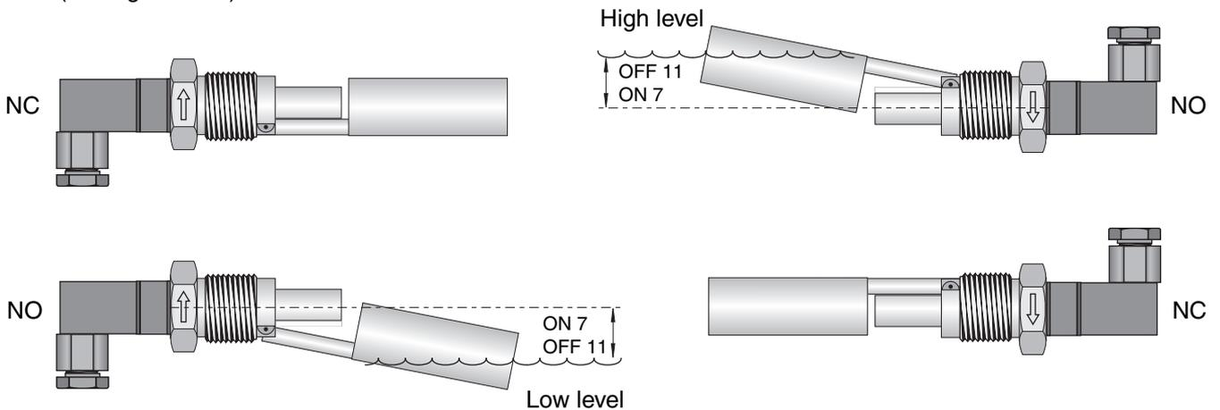
Delivery status of connector is for vertical mounting.
