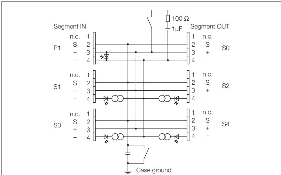
The 4-channel Ex-junction module BBS-48SC-T415B/EX is designed for PROFIBUS-PA systems.
