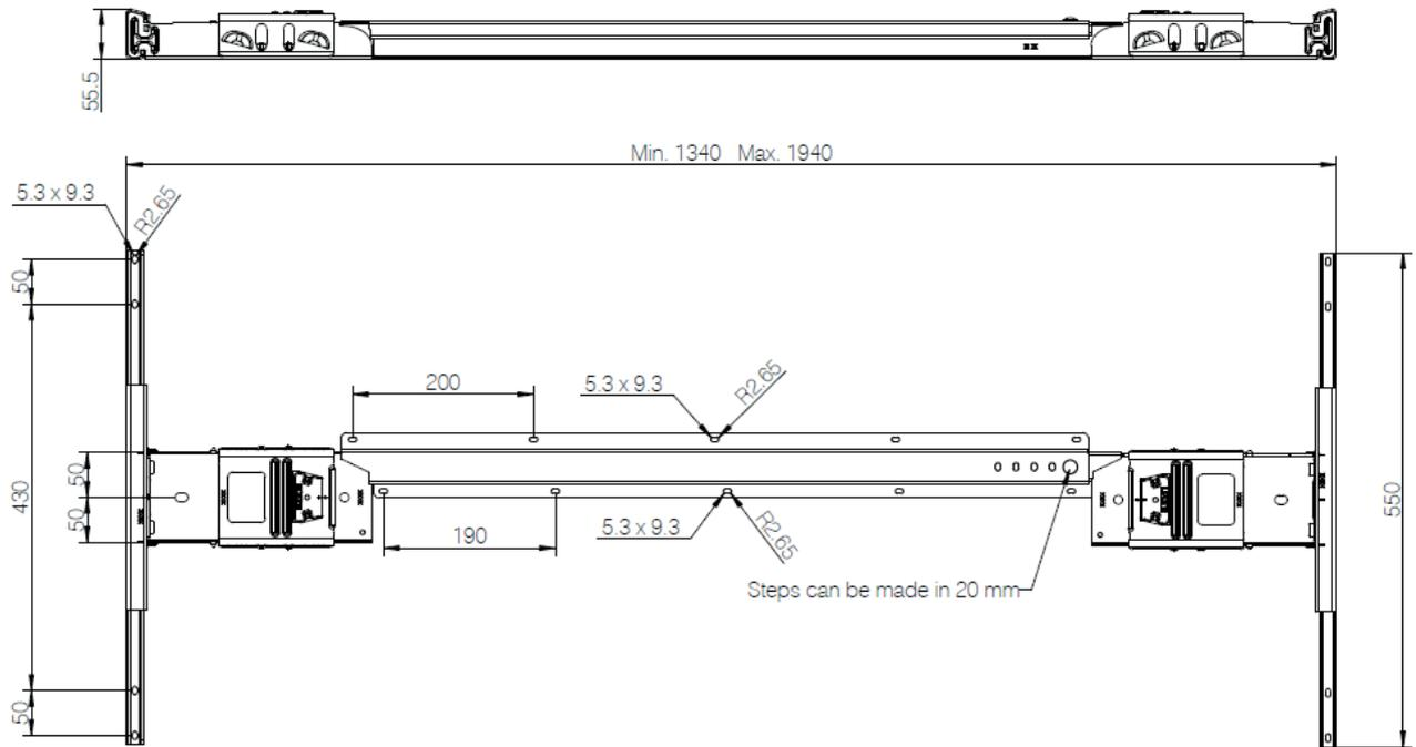
Figure 1 Kick & Click Adjustable dimensions in mm
