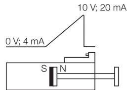
The connector end of the sensor and the north pole of the magnet on the piston must point in the same direction. With all common pneumatic cylinders (e.g. Feso, SMC, Bosch) the north pole shows into to the extension direction of the piston.
