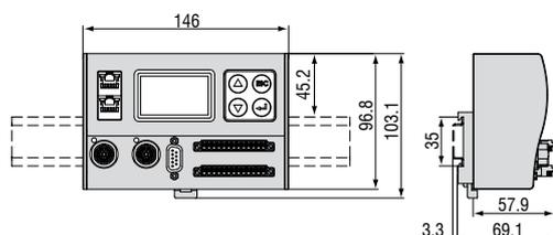
Universal controller with DIN rail TS 35
