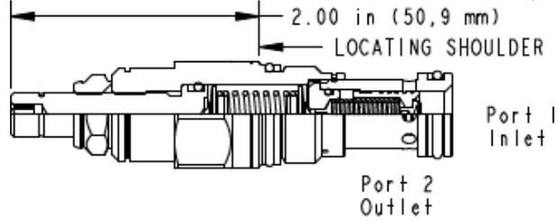
Pilot-operated, balanced-piston relief cartridges are normally closed pressure regulating valves. When the pressure at the inlet (port 1) reaches the valve setting, the valve starts to open to tank (port 2), throttling flow to regulate the pressure. These valves are accurate, have low pressure rise vs. flow, they are smooth and quiet, and are moderately fast.
