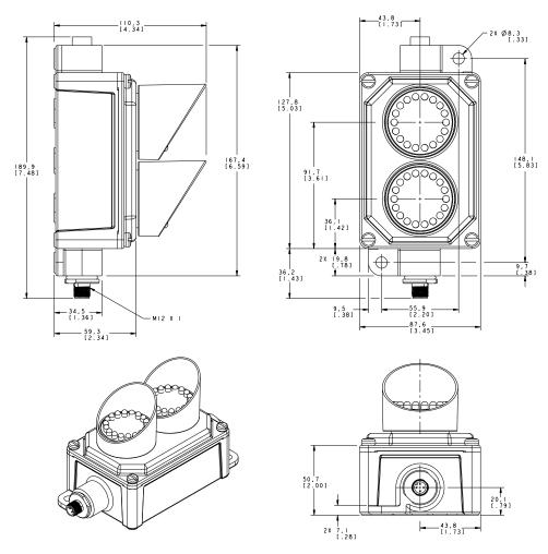
\* Field-wired models have  $\frac{1}{2}$ " NPT port in place of M12 connector
