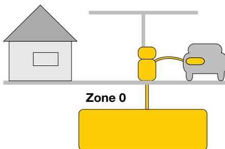
Intrinsically safe devices designed for use in zone 0 must meet category „ia“ safety standards and must have no live contacts. Galvanic isolation between intrinsically safe and non-safe devices is to be preferred. If grounding of the intrinsically safe circuit is required for functionality, this must be done outside zone 0, but as close as possible to zone 0. The devices must as well be approved for gas groups IIA, IIB and IIC.
