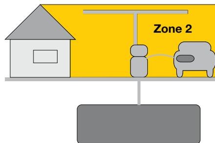
Unlike apparatus for zones 0 and 1, devices for use in zone 2 do not require a test certificate by an authorized body. Devices must conform to category 3 and must meet the following criteria (EN 60079-15):
