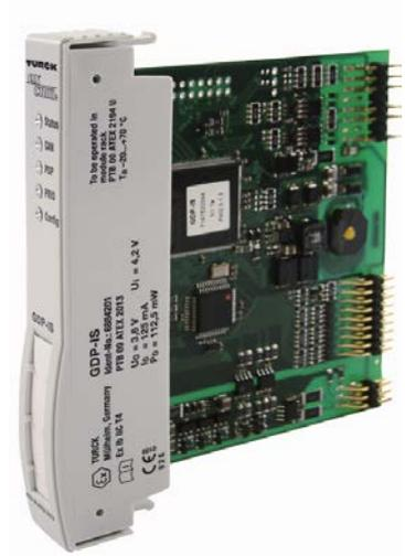
The GDP-IS gateway serves to connect the *excom®* system to PROFIBUS-DP networks. Connection to the PROFIBUS-DP is established via fiber optics or copper cables. The use of fiber optics for data transfer requires the connection of a coupler pair between wired and optical PROFIBUS and also for level adjustment to the IS layer. When using copper cables it is required to install a segment coupler (RS485-IS coupler) to ensure explosion protection.
