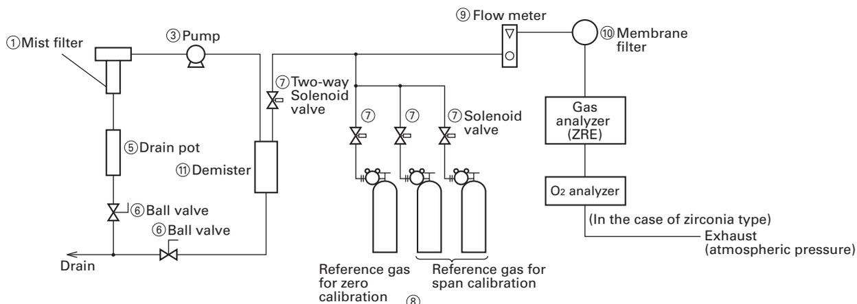
To measure high moisture content sample gas, NO, SO<sub>2</sub>, or CO (0 to 200 ppm range)
