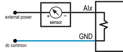
**Analog Input Wiring (4–20mA, 2-Wire, Switch Powered Sensors)**
