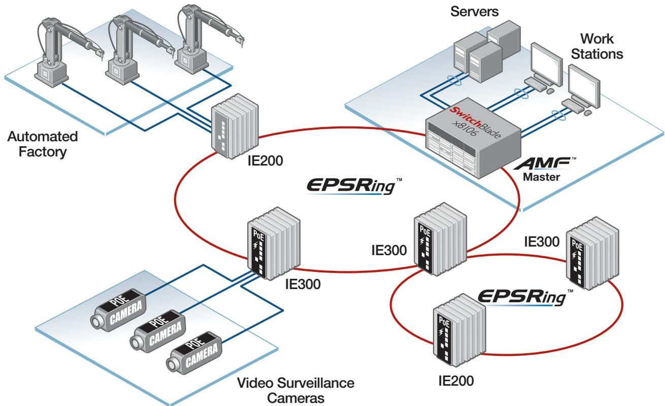
EPSRing™ and ITU-T G.8032 provide high speed resilient ring connectivity. This diagram shows the IE Series in a double ring network topology.
