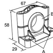
**Hole center spacing:** A=ø 50.8
