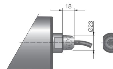
Fig.: Straight hygienic connector, IP69k stainless
