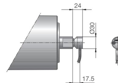
Fig.: Elbow connector, stainless steel
