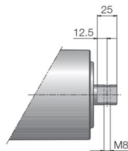
Fig.: Shaft, cross-drilled and threaded
