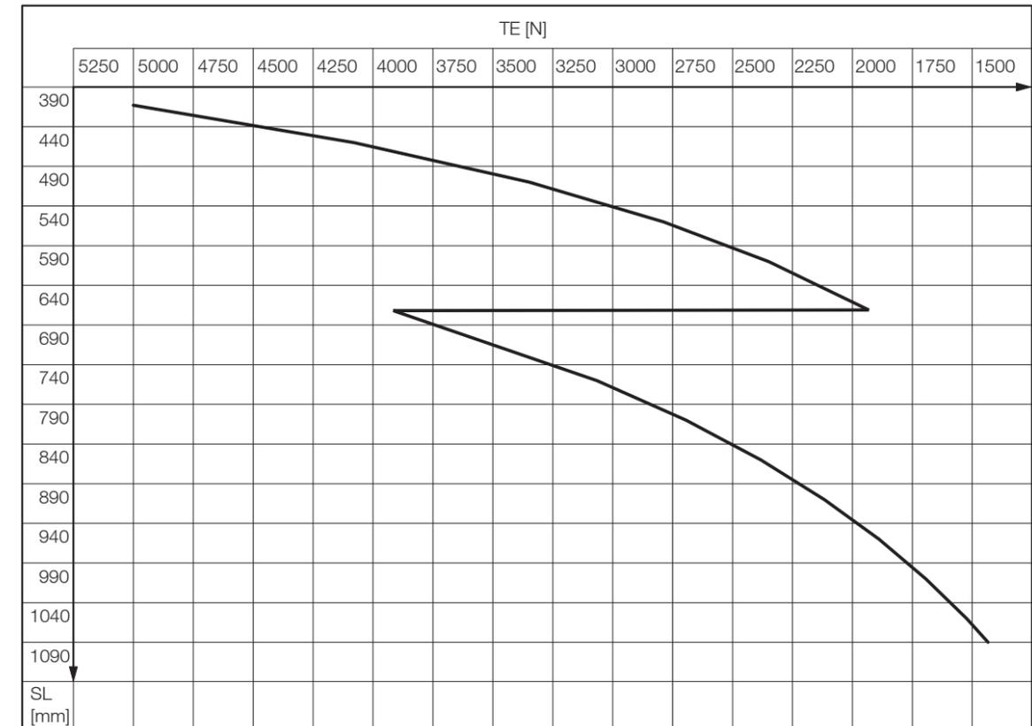
**Note:** To get the right value of the maximum allowed belt tension, first find the maximum allowed TE value for the drum motor RPM. For motors with SL > 400 mm, check if the maximum allowed TE value for the SL is lower. In this case, use the lower value as maximum allowed TE value.
