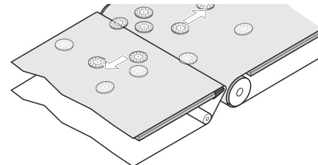
Fig.: Knife-edge conveyor
