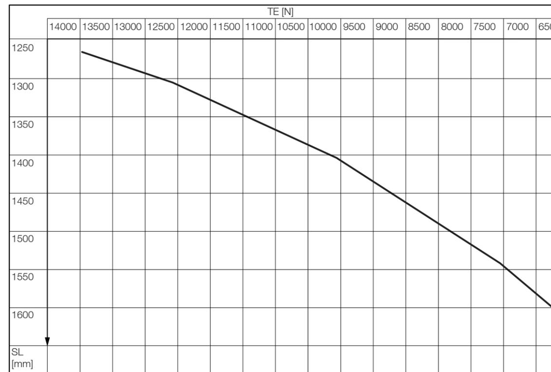
**Note:** To get the right value of the maximum allowed belt tension, first find the maximum allowed TE value for the drum motor RPM. For motors with SL > 1,250 mm, check if the maximum allowed TE value for the SL is lower. In this case, use the lower value as maximum allowed TE value.
