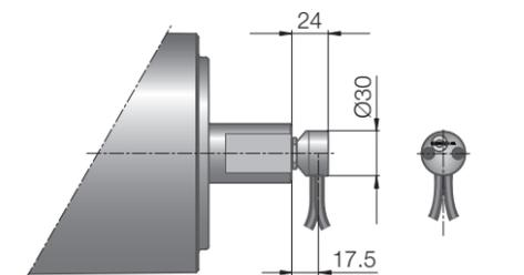
Fig.: Elbow connector / Feedback device,
