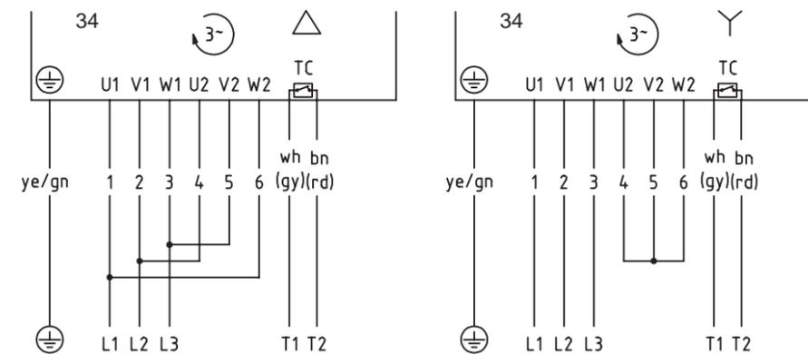
**Fig.: 3-phase operation, 7+2 lead cable, winding for 2 voltages, delta or star connection**
