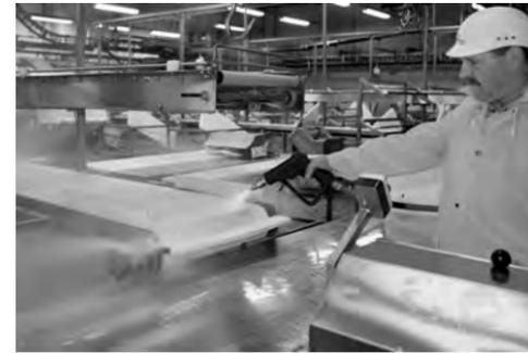
Wet and wash-down applications require rust-free or stainless steel materials for the drum motor shell and the sealing system.
