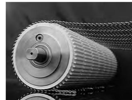
Plastic modular belts, solid homogeneous belts, steel mesh or wire belts are positively driven with no tension. Because the belt has very little direct contact with the drum shell, heat dissipation is less effective and therefore the drum motor should be used in conjunction with a frequency inverter optimised for this application. Alternatively a motor for applications with positive drive belts or no belts, or a synchronous drum motor can be used.
