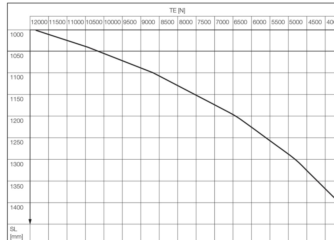
**Note:** To get the right value of the maximum allowed belt tension, first find the maximum allowed TE value for the drum motor RPM. For motors with SL > 1,000 mm, check if the maximum allowed TE value for the SL is lower. In this case, use the lower value as maximum allowed TE value.
