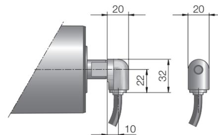
Fig.: Elbow connector, technopolymer
