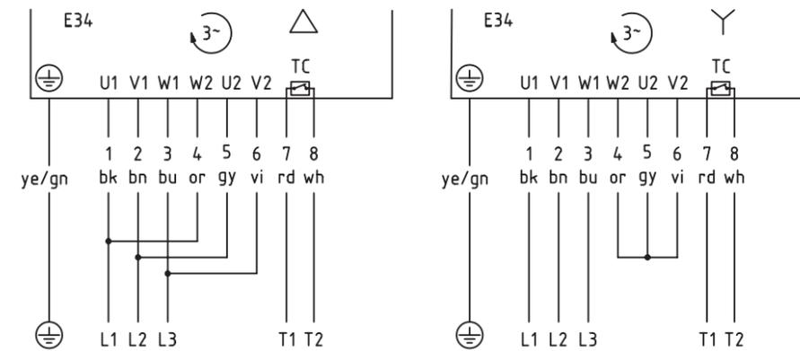
**Fig.: 3-phase operation, 9 lead cable, winding for 2 voltages, delta or star connection**
