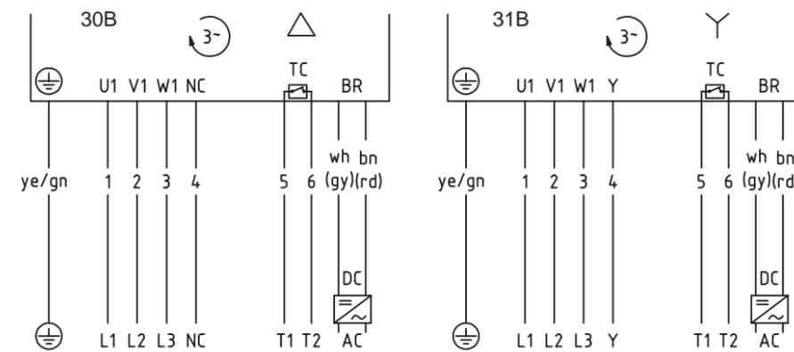
**Fig.: 3-phase operation, 7+2 lead cable, winding for 1 voltage, delta or star connection (internally connected), with brake**
