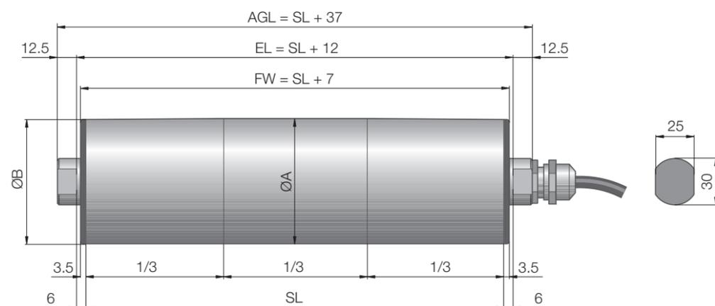
Fig.: Drum motor with straight connector
