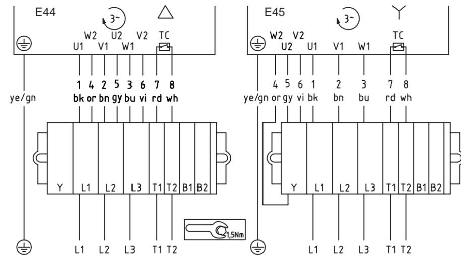
**Fig.: 3-phase operation, 9 lead cable, winding for 2 voltages, delta or star connection**
