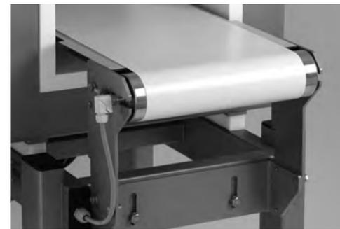
Friction drive belts use the friction between the drum motor shell and belt to drive the belt. The drum motor is normally crowned to prevent belt wander. The belt must be tensioned in order to transmit the torque from the drum motor. The top surface of the belt can be flat, plain or have a ribbed, grooved or diamond pattern.
