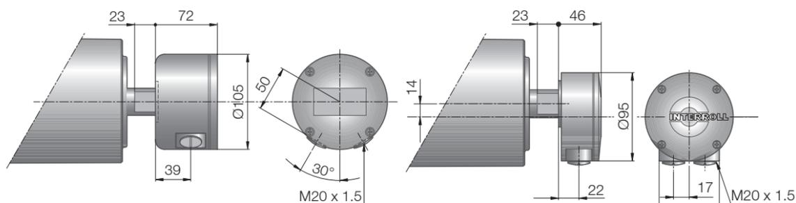
Fig.: Terminal box, technopolymer
