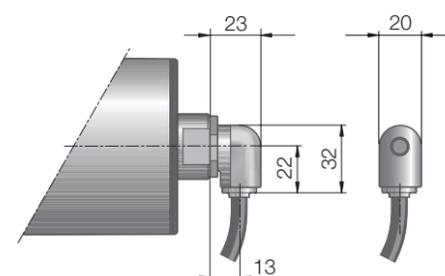
Fig.: Elbow connector, technopolymer
