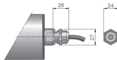
Fig.: Straight connector, brass/nickel or stainless steel
