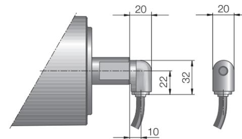
Fig.: Elbow connector, technopolymer
