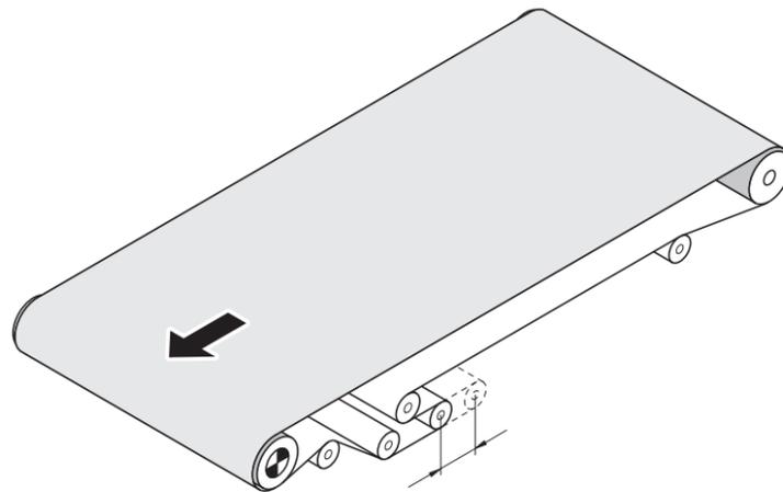
Fig.: Optional design for non-reversible long conveyor with centre take-up
