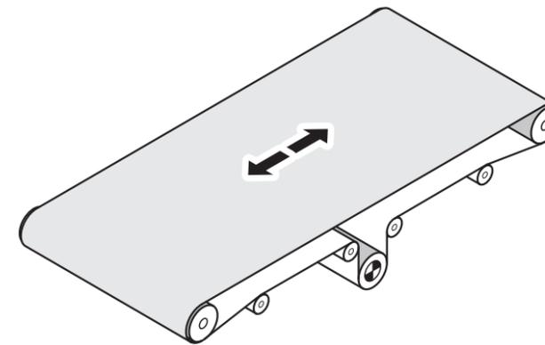
Fig.: Long belt conveyor with centre drive
