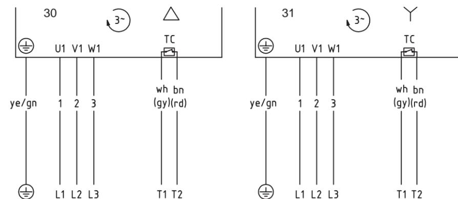
**Fig.: 3-phase operation, 4+2 lead cable, winding for 1 voltage, delta or star connection (internally connected)**
