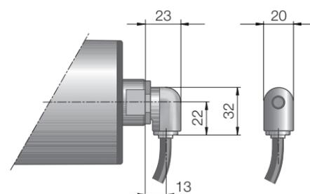
Fig.: Elbow connector, technopolymer
