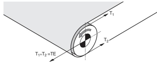
The required belt tension T1 (top side) and T2 (bottom side) can be calculated in accordance with DIN 22101 or CEMA Standard. The actual belt tension can be roughly defined on the basis of the belt manufacturer's specifications by measuring the belt elongation during tensioning.
