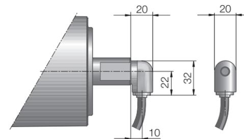
Fig.: Elbow connector, technopolymer
