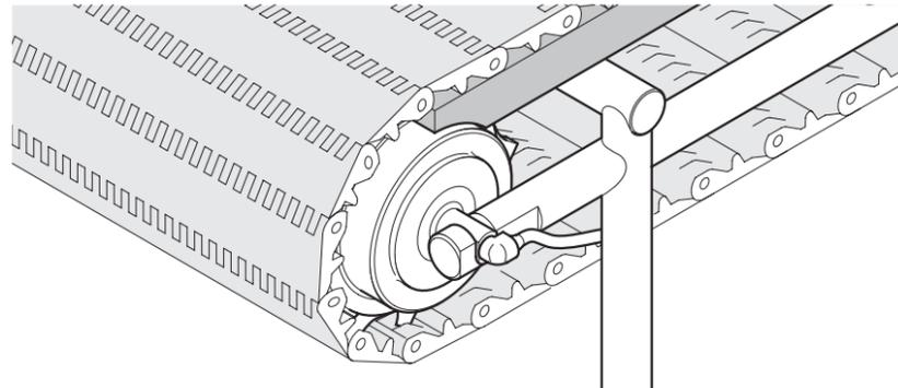
**Fig.:** Open conveyor design for hygienic cleaning
