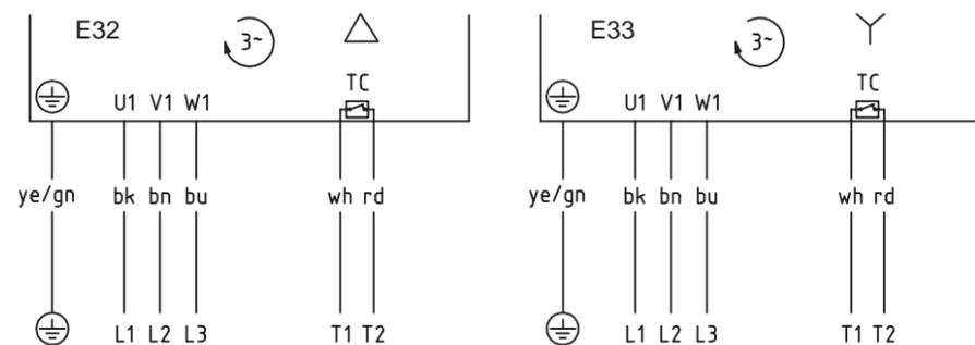
**Fig.: 3-phase operation, 6 lead cable, winding for 1 voltage, delta or star connection (internally connected)**
