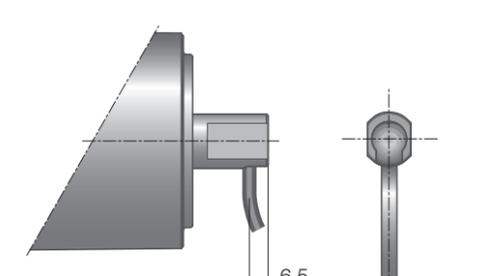
Fig.: Cable slot connector
