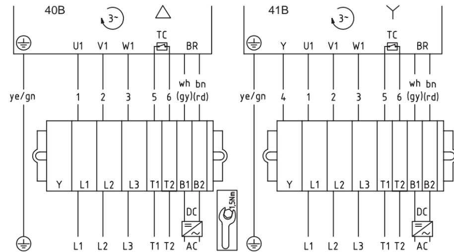
**Fig.: 3-phase operation, winding for 1 voltage, delta or star connection, with brake (internally connected)**
