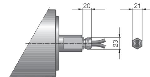
Fig.: Straight connector / Feedback device, brass/
