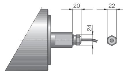
Fig.: Straight connector, stainless steel
