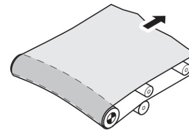
Fig.: Damaged drum motor due to over-tensioning
