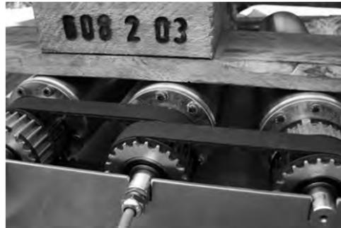
For applications without a conveyor belt or narrow belt, covering less than 70 % of the drum motor face width, heat from the motor cannot be dissipated via the belt contact and therefore asynchronous drum motors must be optimised for applications with positive drive belts or no belts. This can also be done with a frequency inverter. Alternatively a synchronous drum motor can be used.
