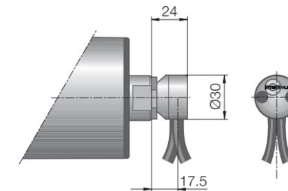
Fig.: Elbow connector / Feedback device, stainless steel
