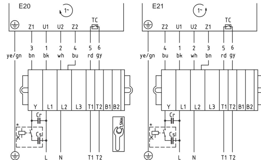
**Fig.: 1-phase operation, 7 lead cable**
