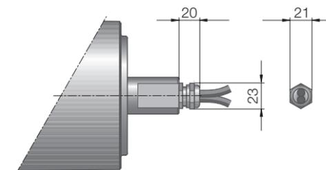
Fig.: Straight connector / Feedback device,
