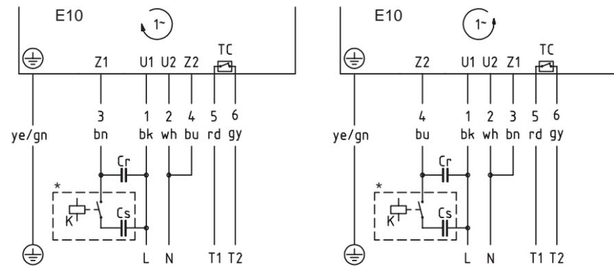
**Fig.: 1-phase operation, 7 lead cable**
