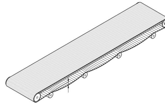
**Fig.: Medium and long conveyor with catenary sags and support rollers on the return belt**
