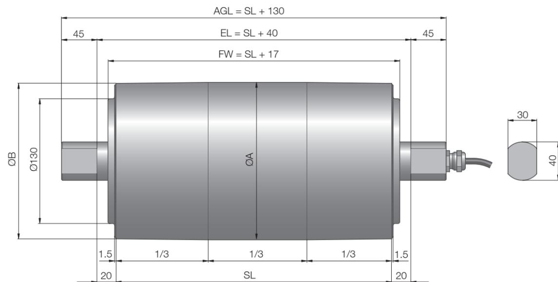
Fig.: Drum motor with straight connector
