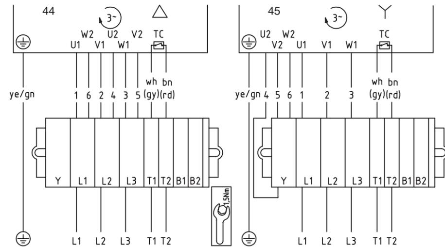
**Fig.: 3-phase operation, winding for 2 voltages, delta or star connection**
