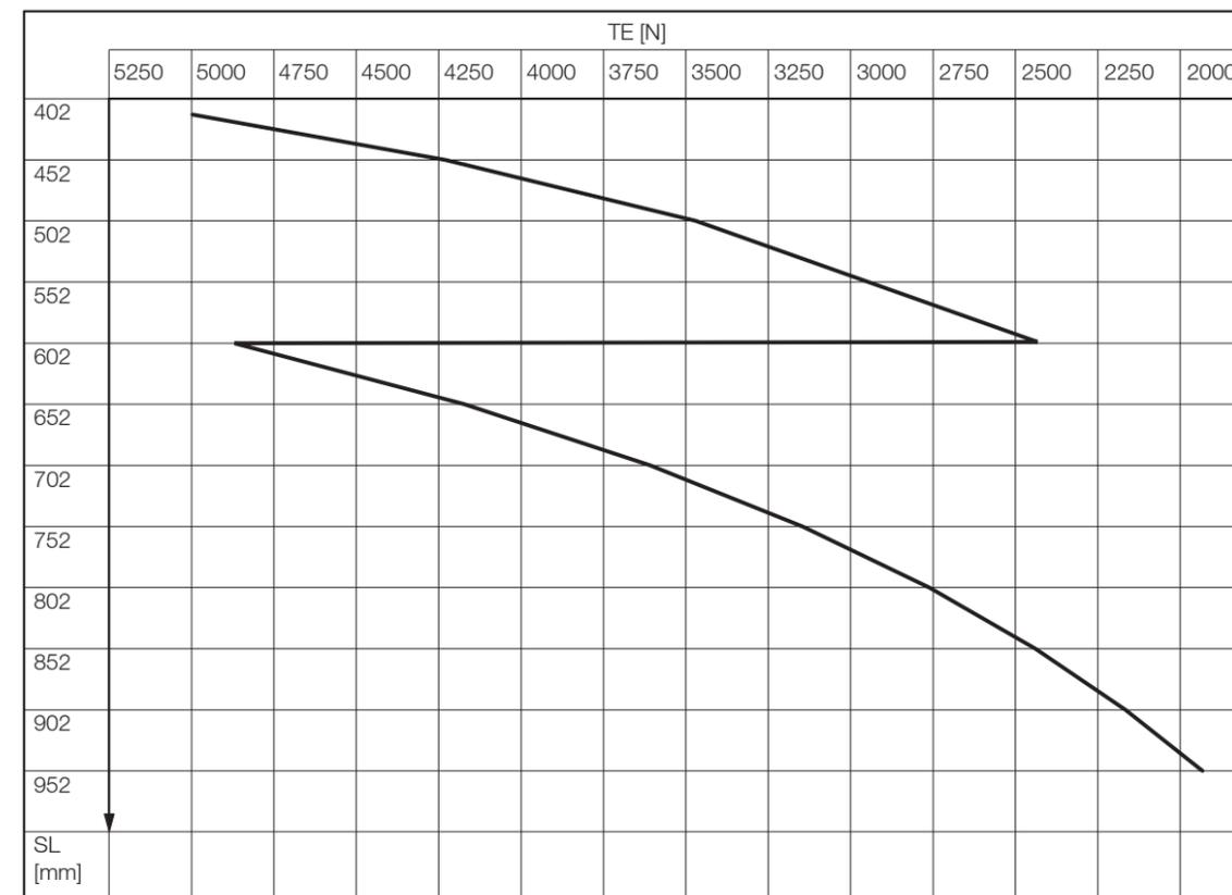
**Note:** To get the right value of the maximum allowed belt tension, first find the maximum allowed TE value for the drum motor RPM. For motors with SL > 402 mm, check if the maximum allowed TE value for the SL is lower. In this case, use the lower value as maximum allowed TE value.
