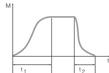
**Fig.:** Closing and opening response time
