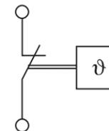
**Fig.: Standard thermal/current overload protection - automatically resetting**
