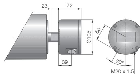
Fig.: Terminal box, technopolymer
