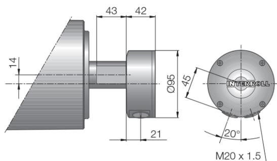
Fig.: Terminal box, stainless steel
