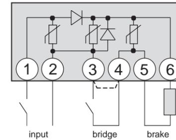
Fig.: Half-wave rectifier
