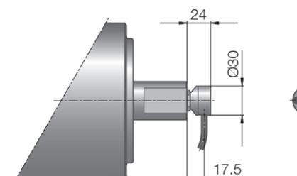
Fig.: Elbow connector, stainless steel
