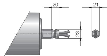
Fig.: Straight connector / Feedback device,
