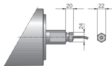
Fig.: Straight connector, stainless steel
