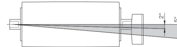
All i-series, D-series and 80S drum motors must be mounted within  $\pm 5^\circ$  of the horizontal. 113S drum motors must be mounted within  $\pm 2^\circ$  of the horizontal.
