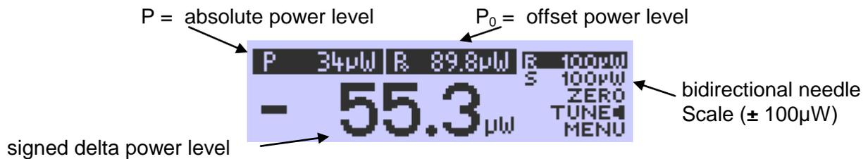
Figure 9 Relative Measurement
