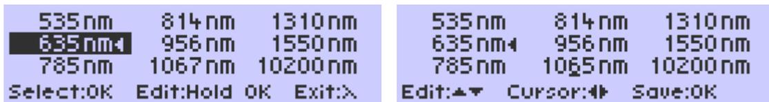
**Figure 6 Wavelength Correction**
