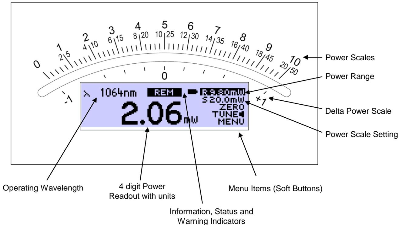
Figure 5 Display Setup
