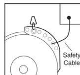
Strongly recommended, secondary steel cable or steel link chain. Prevents balancer from accidental fall. Balancers have extra holes for cable or chain.
