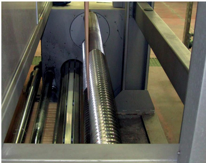
SWS 96 with LG 066 in a rope detwisting device
