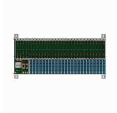
The module rack MT24-3G consists of a backplane and the actual rack system. It can accommodate 2 gateways, 2 power supply units as well as 24 I/O modules. Up to 192 binary inputs/outputs or 96 analog inputs/outputs resp. a mix of both can be connected to it.
