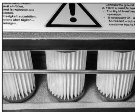
In this case, either the filters or moisture separator is dirty, or the container contains sludge.
