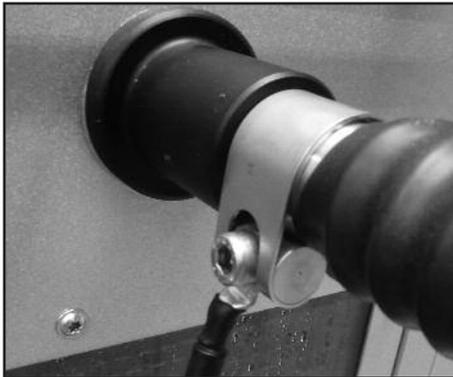
Attach the earthing clip to the metal part of the suction connection.
