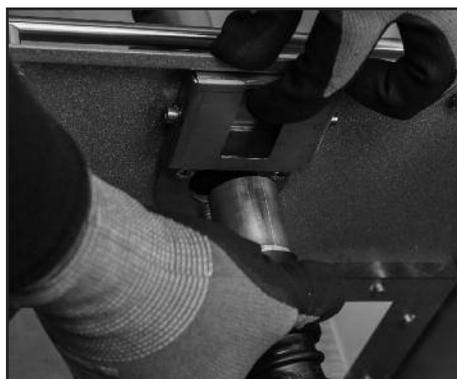
The shut-off valve in the liquid container avoids the possibility that after the container has been cleaned an attempt may be made to run the suction unit without reinstalling the swirl filter.
