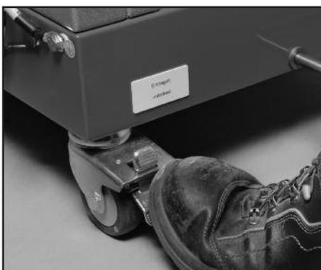
Apply the parking brake (if fitted) to prevent the wet separator from rolling away.
