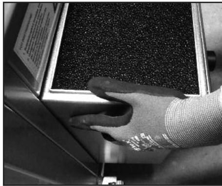
Carefully lift the housing of the moisture separator.
