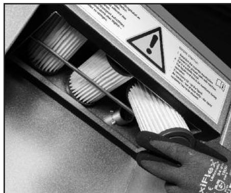
To do this, simply remove the filter cartridges and dispose of them in accordance with environmental regulations.
