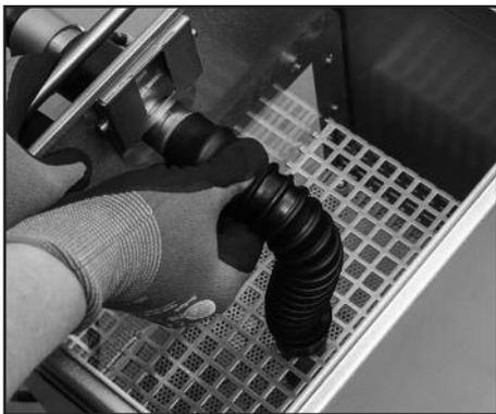
Pulling out the hose automatically activates the shut-off valve, thereby closing the suction connection.
