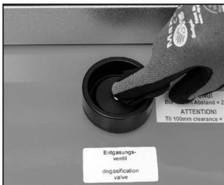
The degasification valve should always be checked for correct operation before commissioning and each time before starting the wet separator. Ensure that the machine is switched off before carrying out this check. The valve head should slot into place with gentle pressure and automatically return to its original position with the help of the spring.
