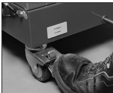
Switch off the wet separator and apply the parking brake - if fitted.
