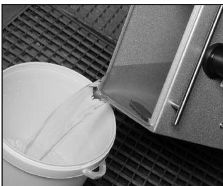
The contents of the container should be emptied out into a suitable vessel. Dispose of the vacuumed material in accordance with all applicable, national environmental regulations
