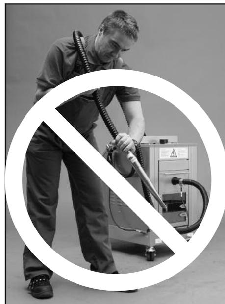
**Avoid any bodily contact with the hose - even during the suction process.**
