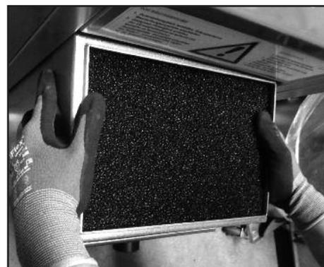
If despite being cleaned the moisture separator is still dirty it must be replaced. Remove the moisture separator from the housing. Then insert a new moisture separator.
