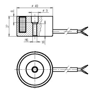
FEATURES – Series of solenoids with zinc plated steel body. Class F insulation (155°C) with class H wire (180°C). Solenoid complying with VDE 0580 directive and 100% inspected.
