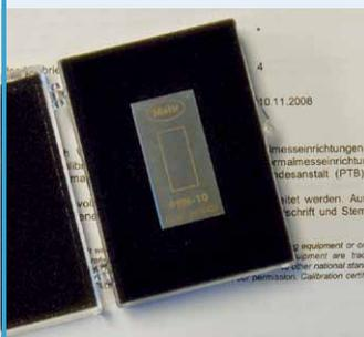
With Mahr calibration certificate. Roughness standard with turned profile, chromed. Profile depth ca. 10  $\mu\text{m}$  (.394  $\mu\text{inch}$ ), for checking the roughness measuring station.
