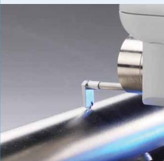
System Single-skid pick-up with lateral, spherical skid
