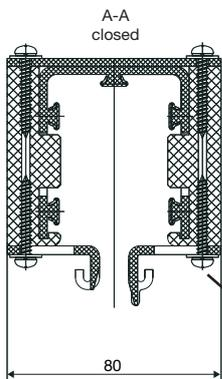
To open the section loosen 4 cross-head screws and push both sliders outwards.
