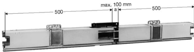
Expansion joint sections are required to compensate expansions and contractions of KSL Powerail in varying temperatures without interrupting electrical power.
