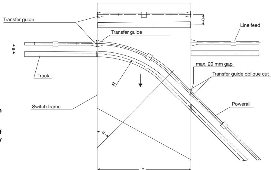
Max. 20 mm air gap between transfer guides.
