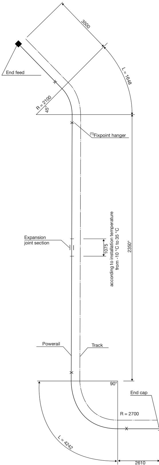
(1) Rest of powerail to be installed with sliding hangers
