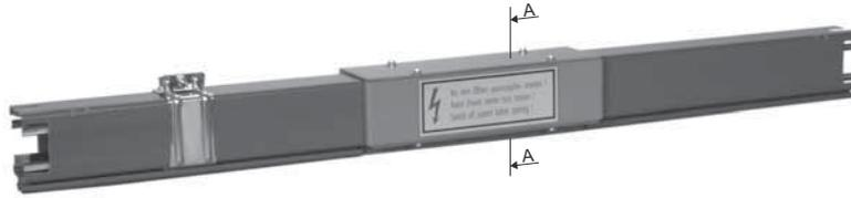
Assembly and disassembly of the collector is possible at the end of the track as well as at the removing section.
