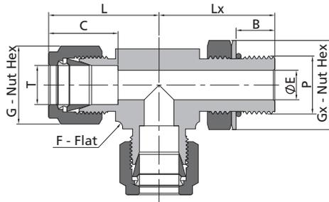
1. The E dimension refers to the smallest nominal orifice. It might be larger at tapered thread end, straight thread end.
