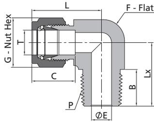
The E dimension refers to the smallest nominal orifice. It might be larger at tapered thread end, straight thread end.
