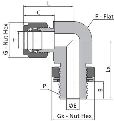
The E dimension refers to the smallest nominal orifice. It might be larger at tapered thread end, straight thread end.
