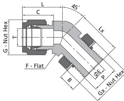
1. The E dimension refers to the smallest nominal orifice. It might be larger at tapered thread end, straight thread end.
