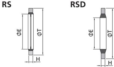
The RS and RSD gaskets provide a seal with male ISO parallel threads. The gasket consists of a fluorocarbon FKM or Buna inner ring bonded to a carbon steel or stainless steel outer ring.
