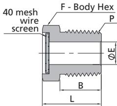
40 mesh 300 series stainless steel wire screen assembly
