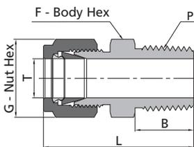
1. The T dimension refers to the smallest nominal orifice. It might be larger at tapered thread end, straight thread end.
