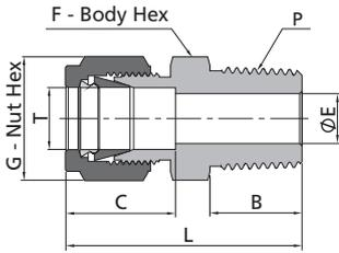
The E dimension refers to the smallest nominal orifice. It might be larger at tapered thread end, straight thread end.
