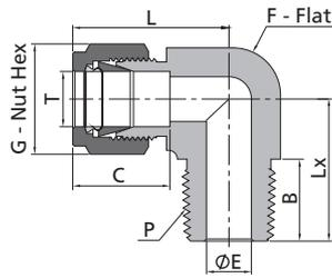
The E dimension refers to the smallest nominal orifice. It might be larger at tapered thread end, straight thread end.
