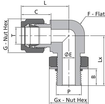
1. The E dimension refers to the smallest nominal orifice. It might be larger at tapered thread end, straight thread end.
