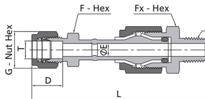
The E dimension refers to the smallest nominal orifice. It might be larger at tapered thread end, straight thread end.
