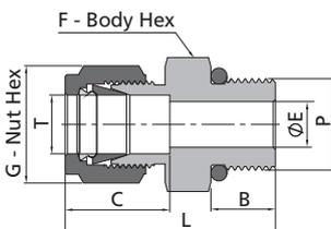
1. The E dimension refers to the smallest nominal orifice. It might be larger at tapered thread end, straight thread end.
