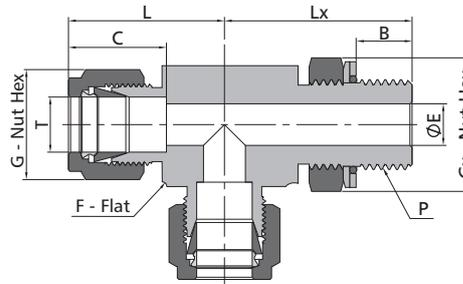
The E dimension refers to the smallest nominal orifice. It might be larger at tapered thread end, straight thread end.
