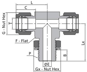
The E dimension refers to the smallest nominal orifice. It might be larger at tapered thread end, straight thread end and welding end.
