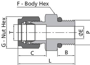
1. The E dimension refers to the smallest nominal orifice. It might be larger at tapered thread end, straight thread end.
