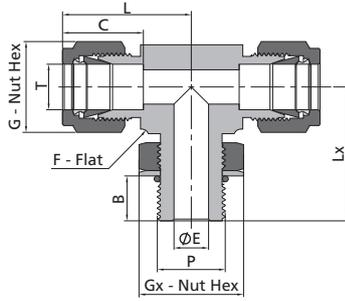
1. The E dimension refers to the smallest nominal orifice. It might be larger at tapered thread end, straight thread end.
