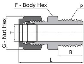
The T dimension refers to the smallest nominal orifice. It might be larger at tapered thread end, straight thread end.
