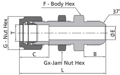
The E dimension refers to the smallest nominal orifice. It might be larger at tapered thread end, straight thread end.
