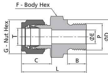
The E dimension refers to the smallest nominal orifice. It might be larger at tapered thread end, straight thread end.
