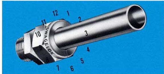
3. Hold the fitting body steady with a backup wrench and tighten the nut 1/4 turns. Watch the scribe mark, make one complete revolution and continue to the 9 o'clock position. When the nut is tightened to the 9 o'clock position, you can easily see the fitting has been tightened properly.
