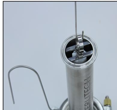
Photo 8: Stir Bar Insertion with Stir Bar Retriever
